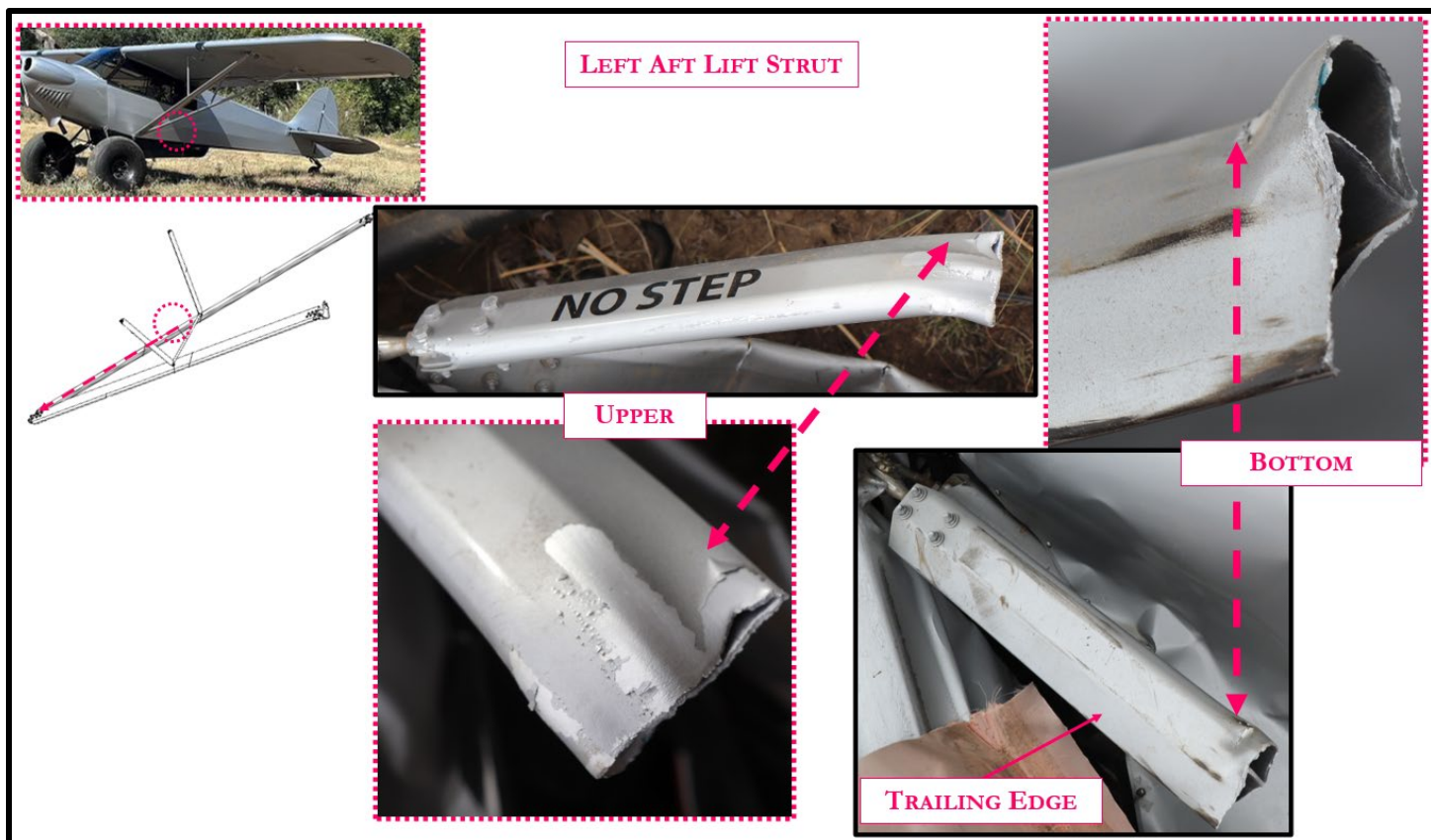
Figure 18: Left aft strut (lower portion)
