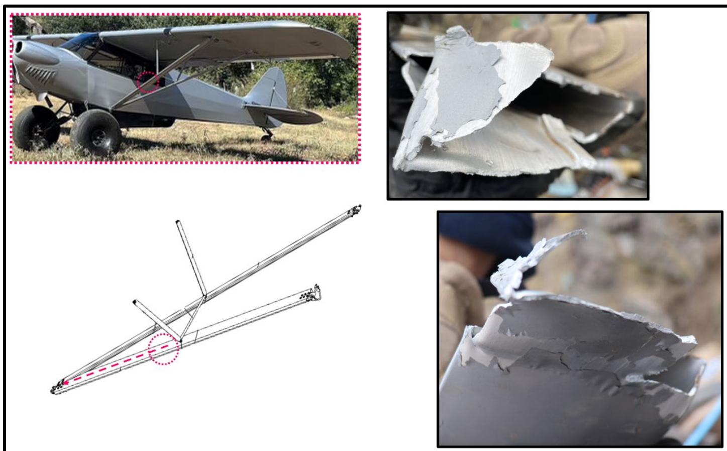
Figure 19: Left forward strut (lower portion)
