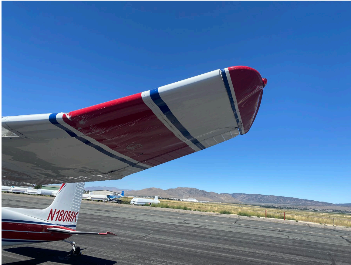
Photograph 2 - Close-up View of Damaged Left Wing (Courtesy of FAA)
