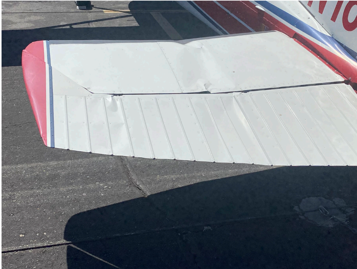
Photograph 3 - Rear View of Damaged Left Horizontal Stabilizer (Courtesy of FAA)
