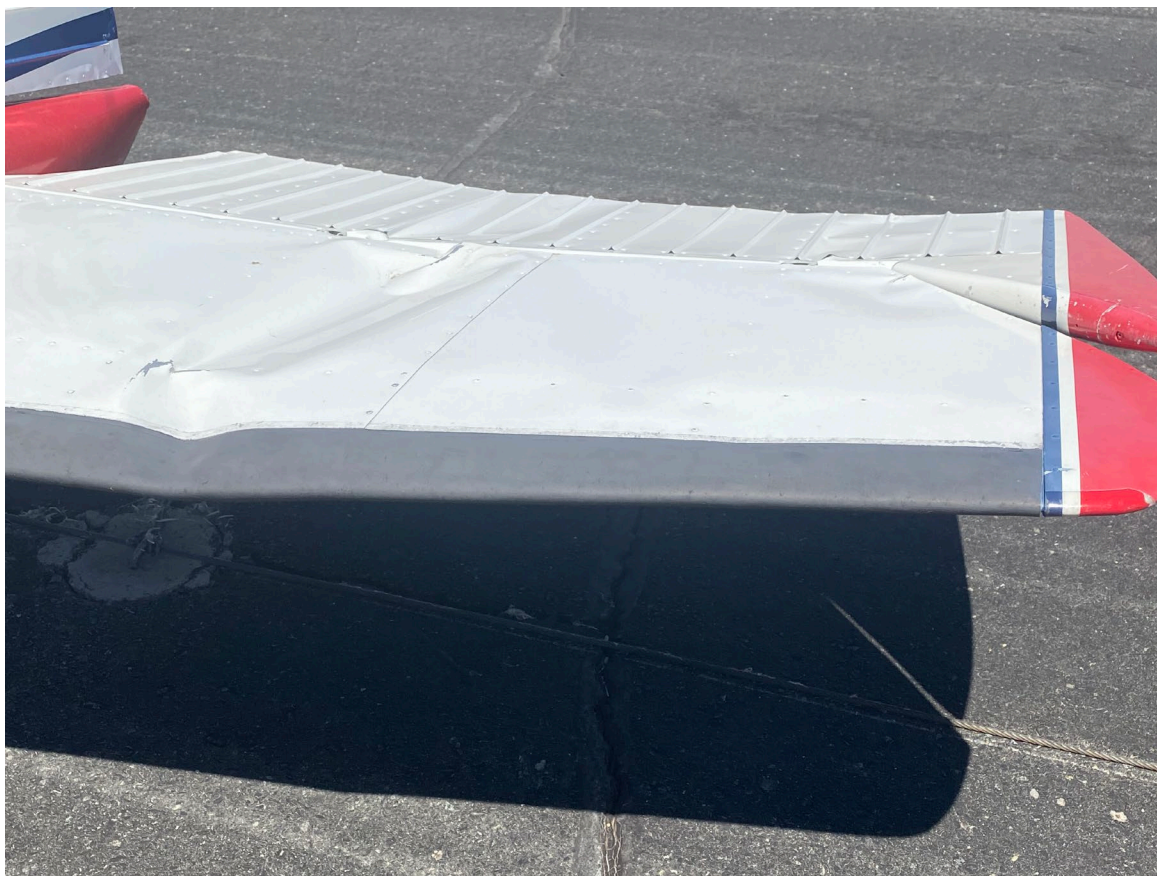
Photograph 4 - Front View of Damaged Left Horizontal Stabilizer (Courtesy of FAA)
