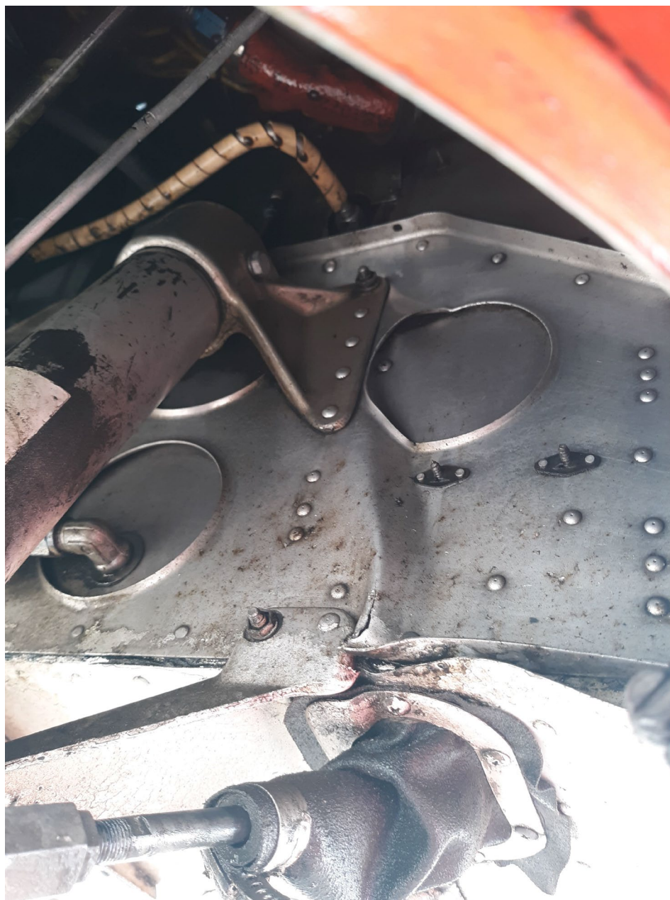
Photo 2 – Damage to the fuselage. Photo courtesy of the FAA.
