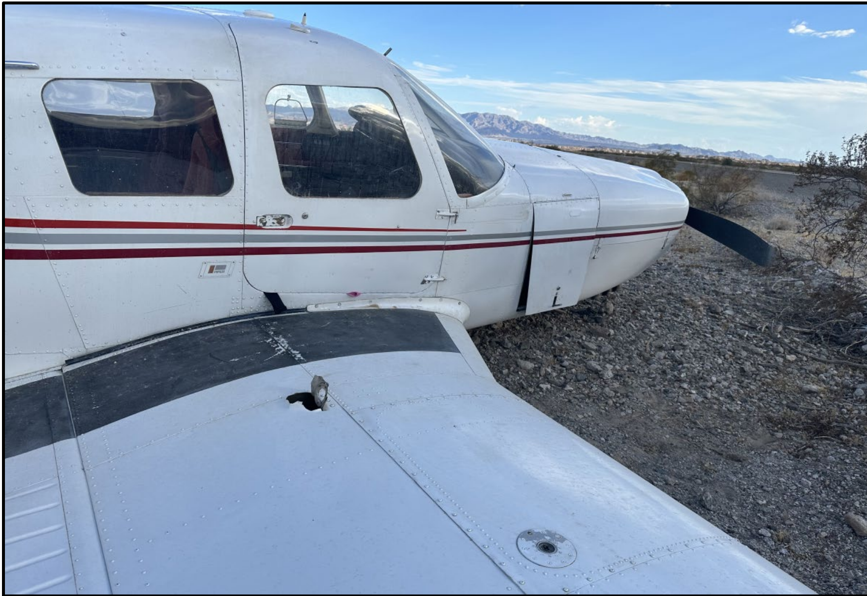
Figure 2: Right Wing with Hole from Landing Gear
