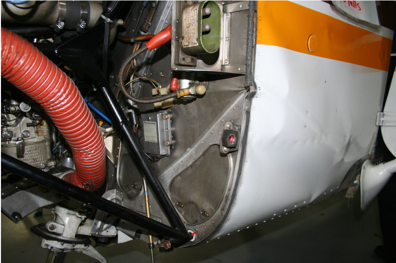
Photograph 1 - View of lower left fuselage damage (Courtesy of repair station)
