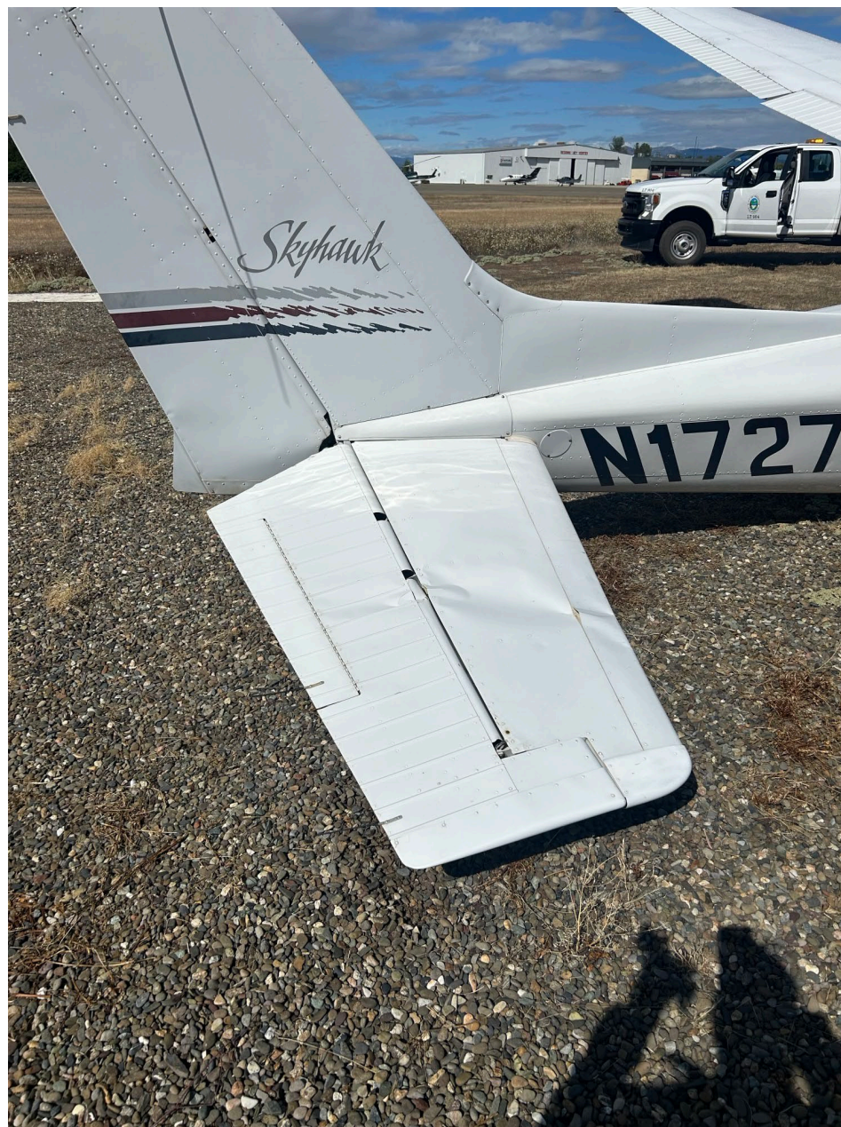
Photo 2 - View of right horizontal and elevator damage (photo courtesy of the witness)
