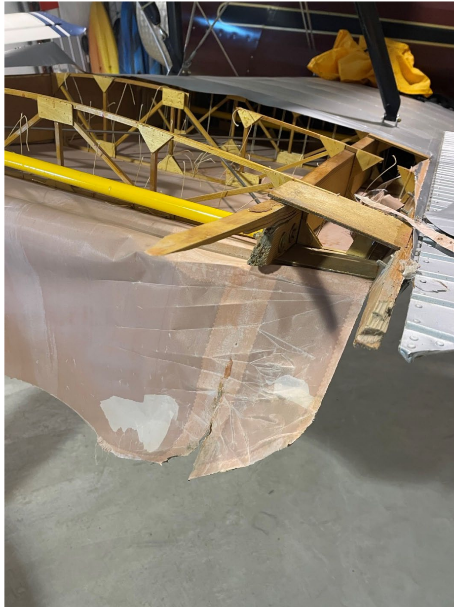
Photo 2 – View of substantial damage to the lower left wing spar (Courtesy of Operator)
