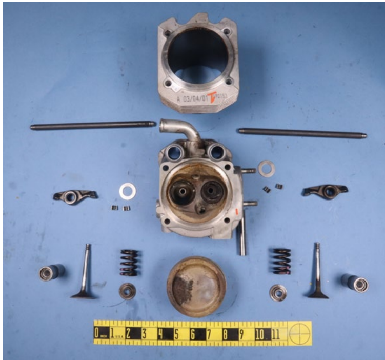
Figure 1. Cylinder 1 components; intake components on the left side of the image, and exhaust components on the right.
