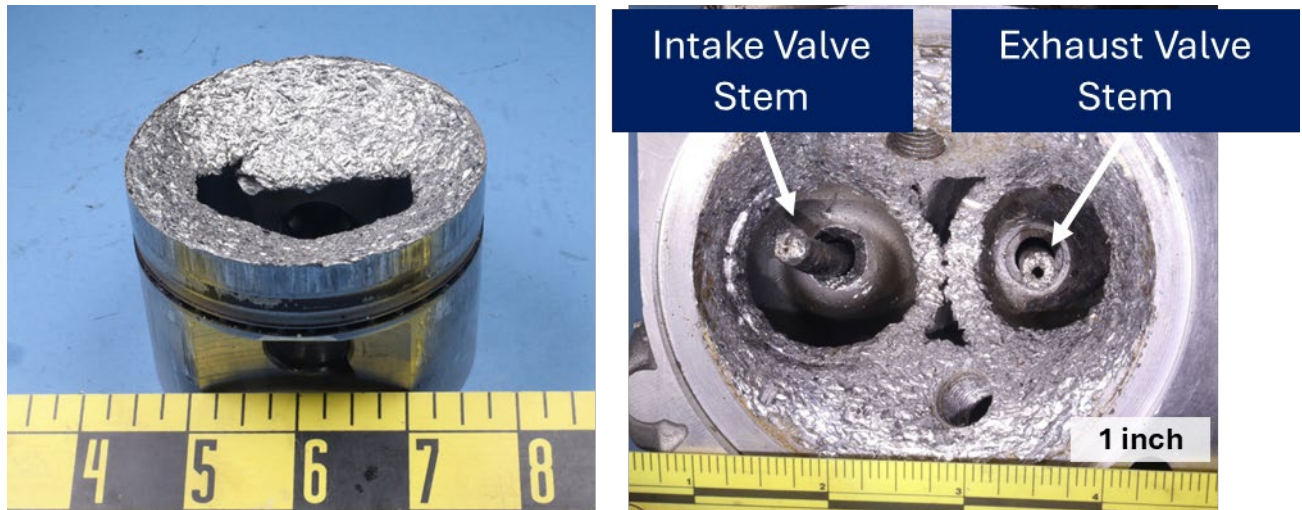
Figure 11. (Left) The piston and (right) cylinder head from cylinder 4 showed significant impact damage across their faces. The fracture surfaces of the valve stems showed similar damage.
