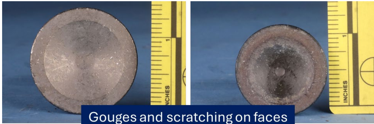
Figure 9. Both the (left) intake and (right) exhaust valves from cylinder 2 showed small gouges and scratches across their faces.
