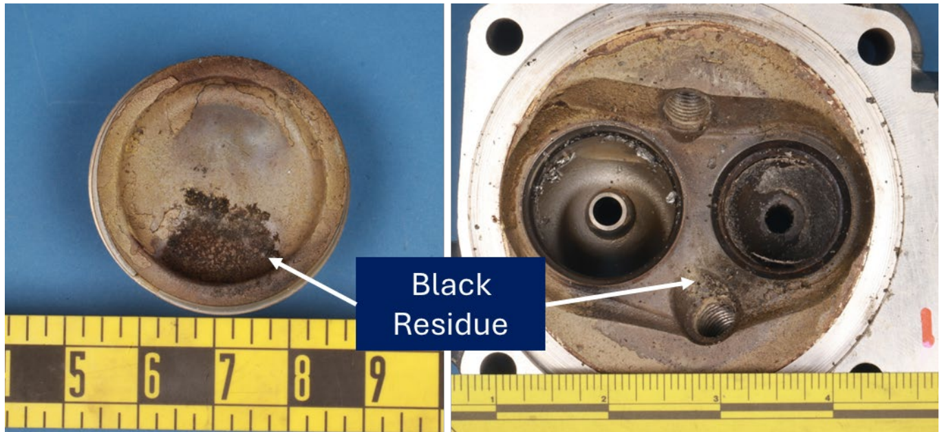
Figure 7. Black residue on the (left) piston and (right) cylinder head for cylinder 1.
