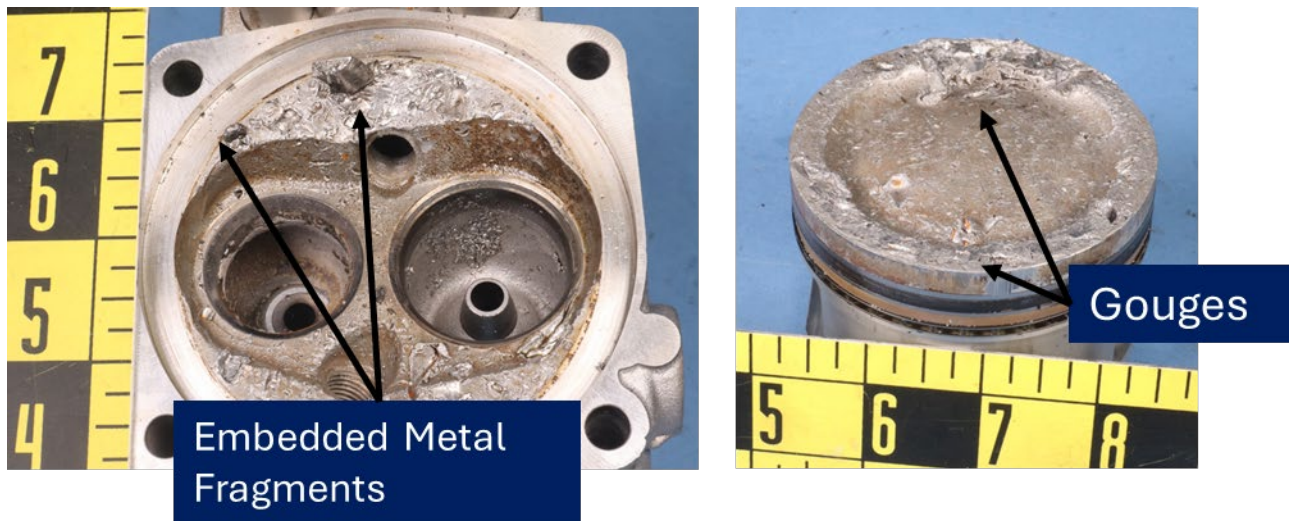
Figure 8. (Left) The cylinder head and (right) piston for cylinder 2 showed gouges across the surfaces. Metal fragments were embedded in the cylinder head.
