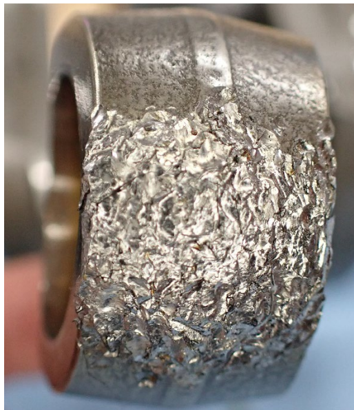
Figure 15: Cylinder 4 connecting rod damaged bushing
