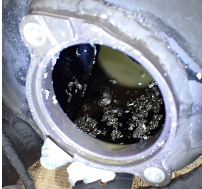
Figure 18: Metallic fragments inside airbox
