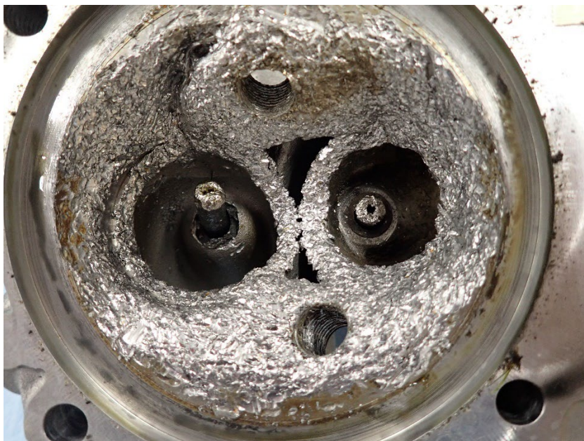
Figure 3: No. 4 interior cylinder head and valve stems
