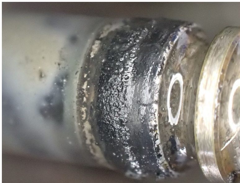
Figure 7: Closeup of black hardened material on upper portion of exhaust valve stem below keeper
