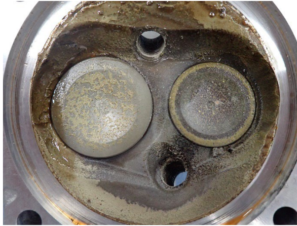
Figure 10: No. 1 cylinder head and valve faces
