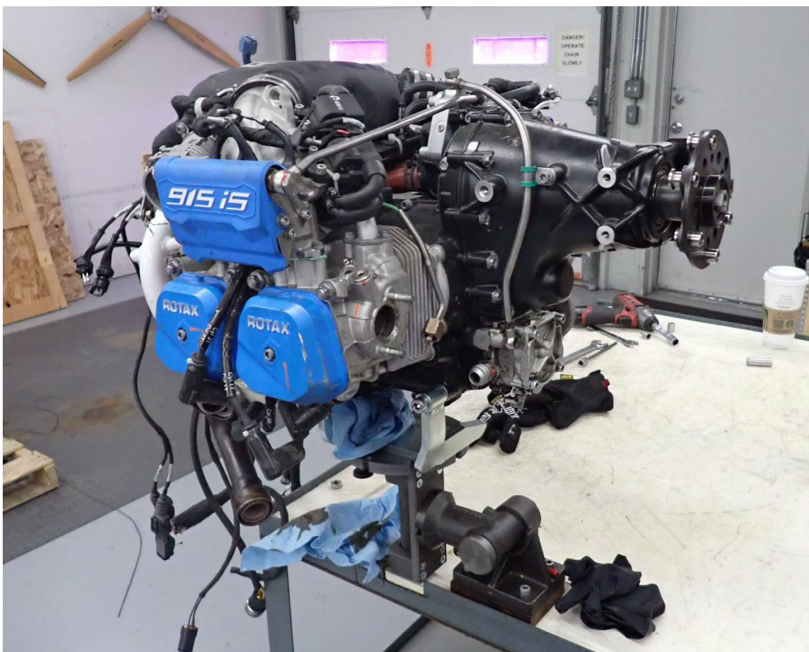
Figure 1: Engine on mount with firewall and engine mount removed
