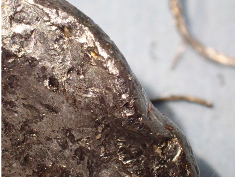
Figure 4: Intake valve face circumference with deformation and gouge markings
