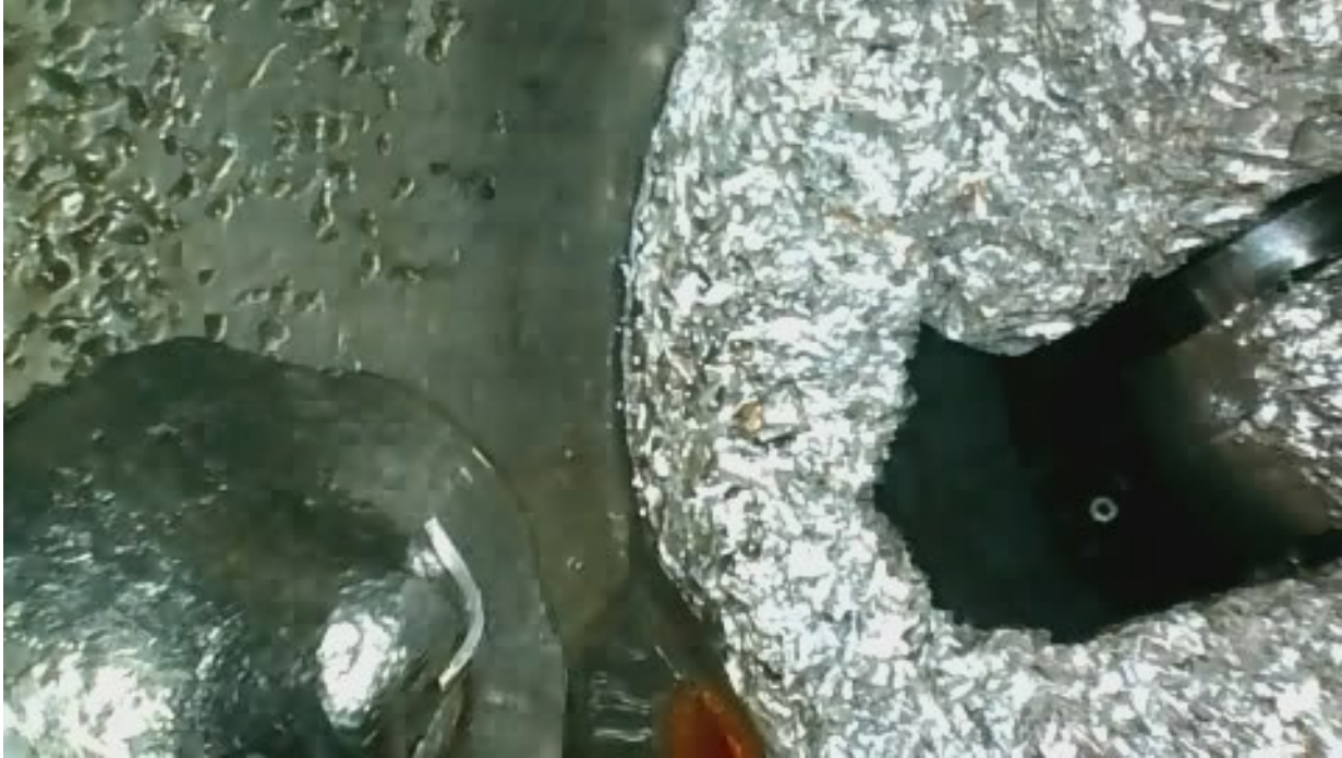
Figure 4: Cylinder 4 pitting on cylinder wall, penetrated piston face, and broken exhaust valve
