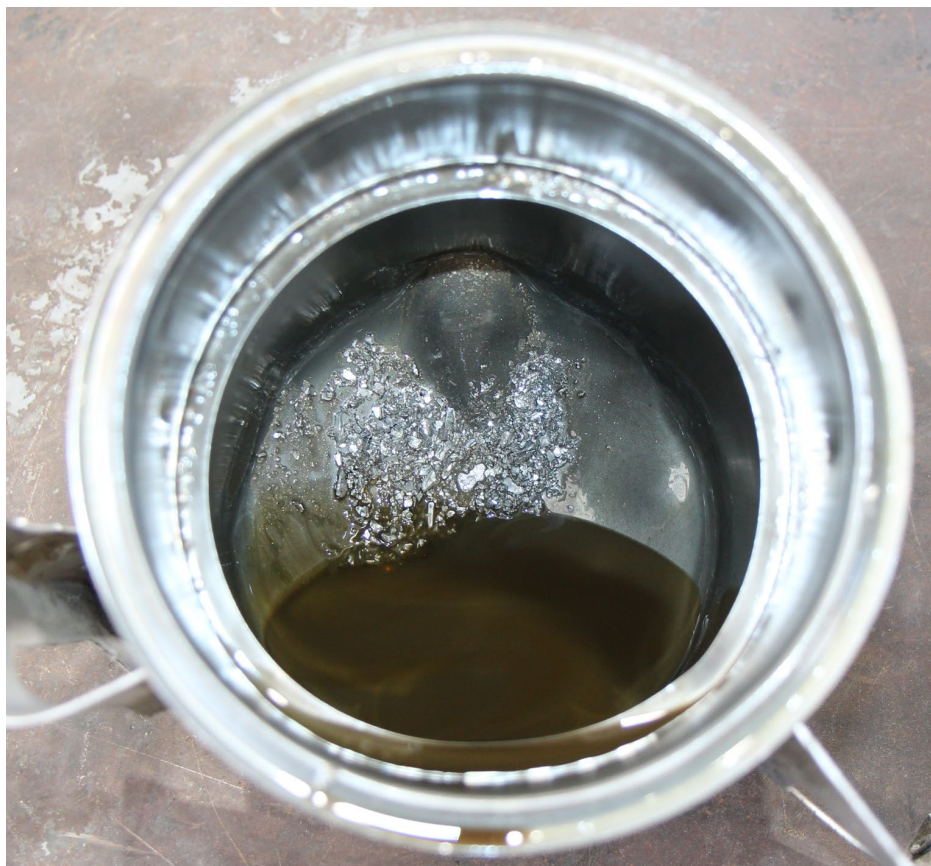
Figure 2: Metallic fragments and bottom of oil sump
