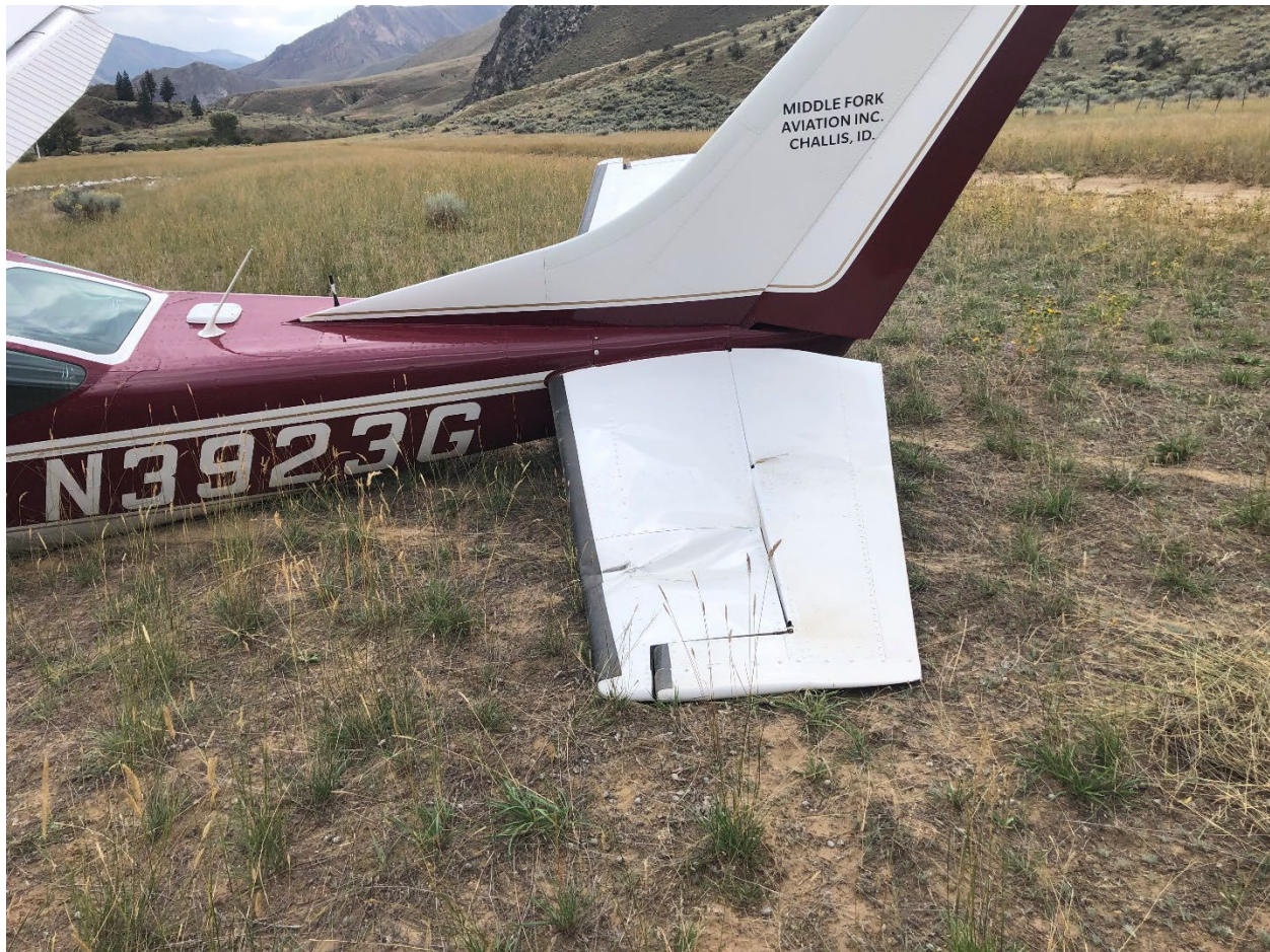
Figure 1. Substantial damage to the left horizontal stabilizer and elevator. Photo courtesy of the pilot.
