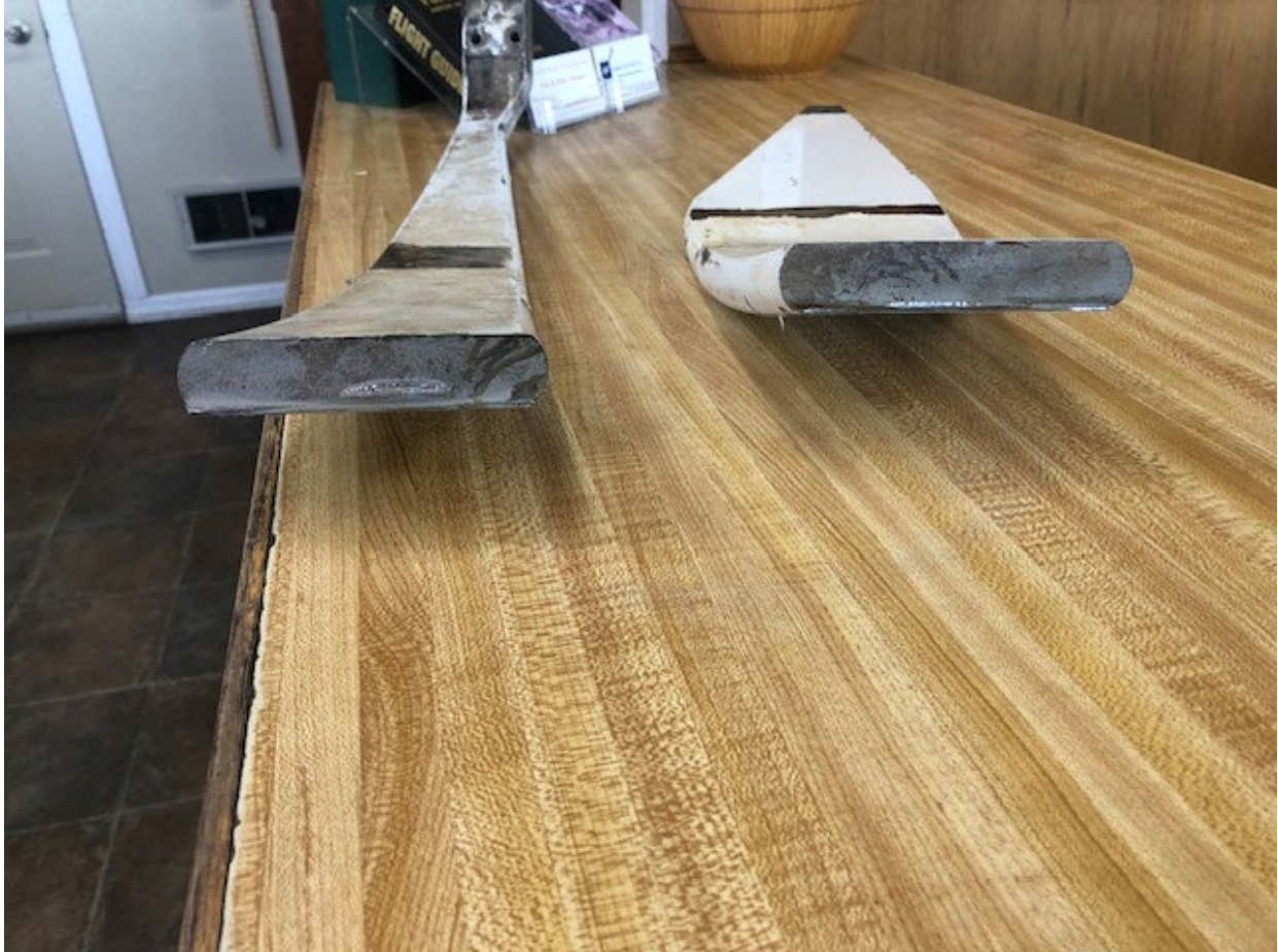
Figure 4. View of the fractured surface of the left main gear spring assembly. Photo owner.
