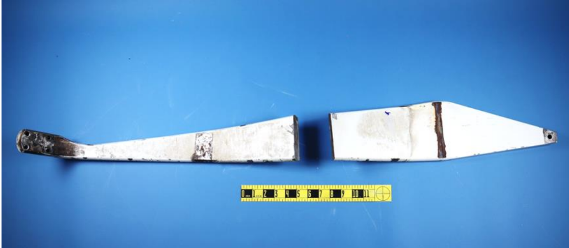
Figure 1. Left landing gear leg as-received.
