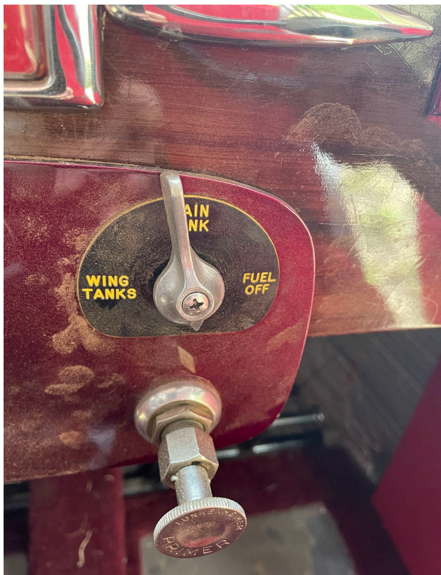
Photograph 2 -View of fuel selector valve pointer positions (photo courtesy of FAA inspector)
