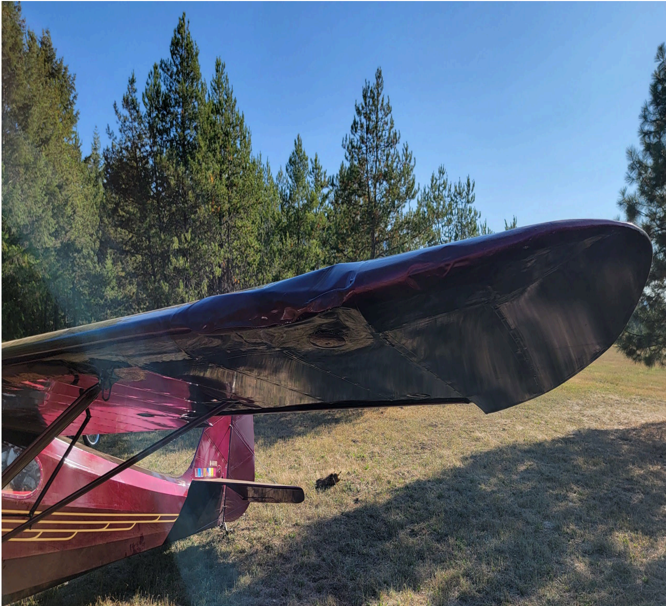
Photograph 1 - View of damage to left wing (photo courtesy of law enforcement officer)
