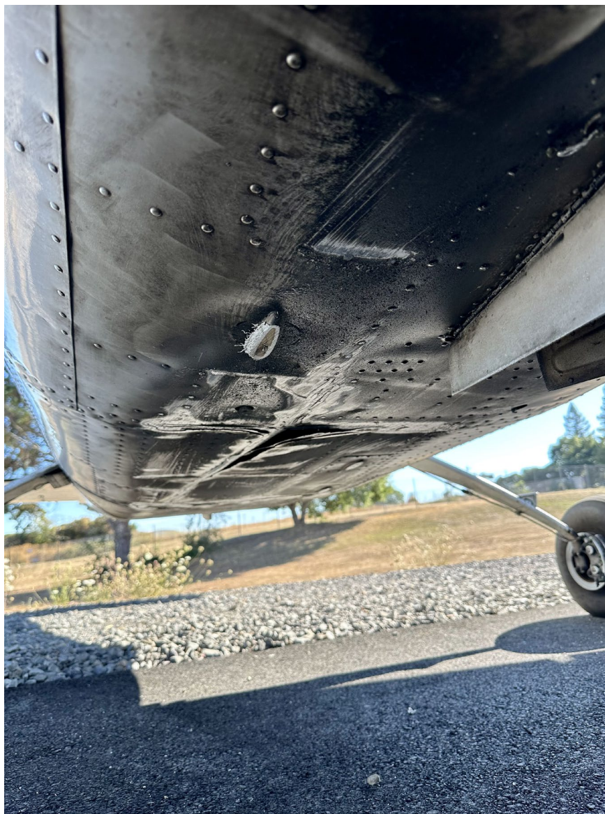
Photograph 2 - Airplane damage (Courtesy of STS Ops)
