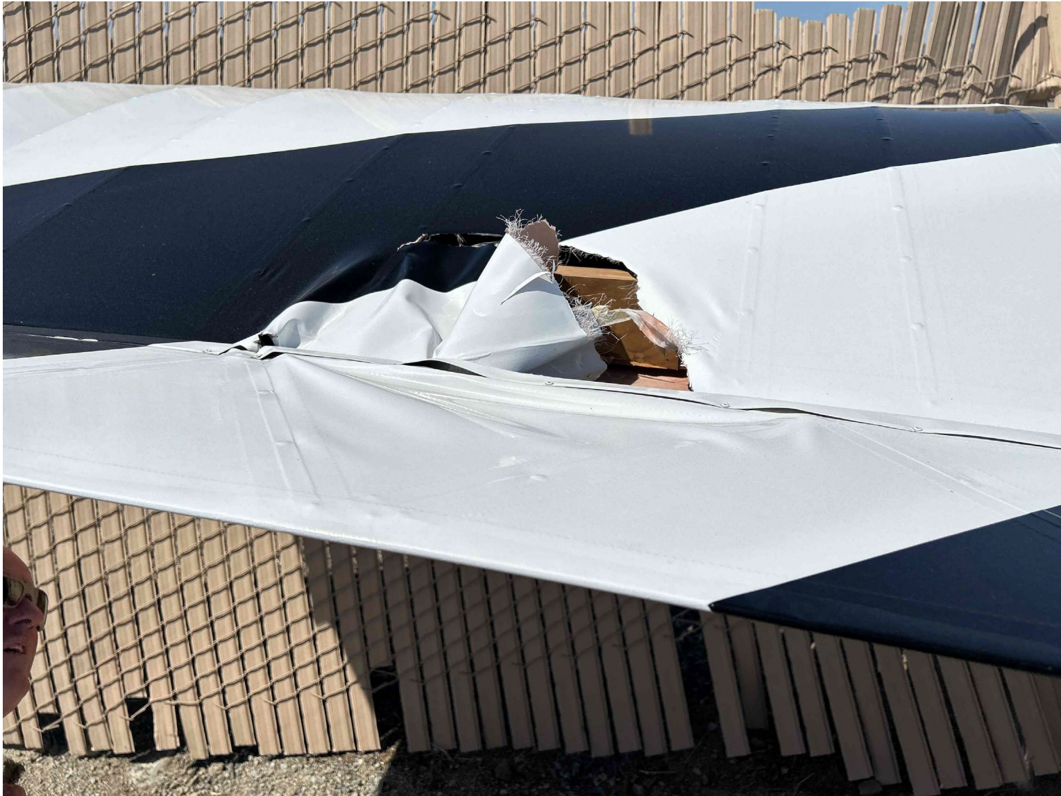
Photograph 1 - Airplane's left wings damage as viewed from the rear. (Courtesy of Airport Operations)
