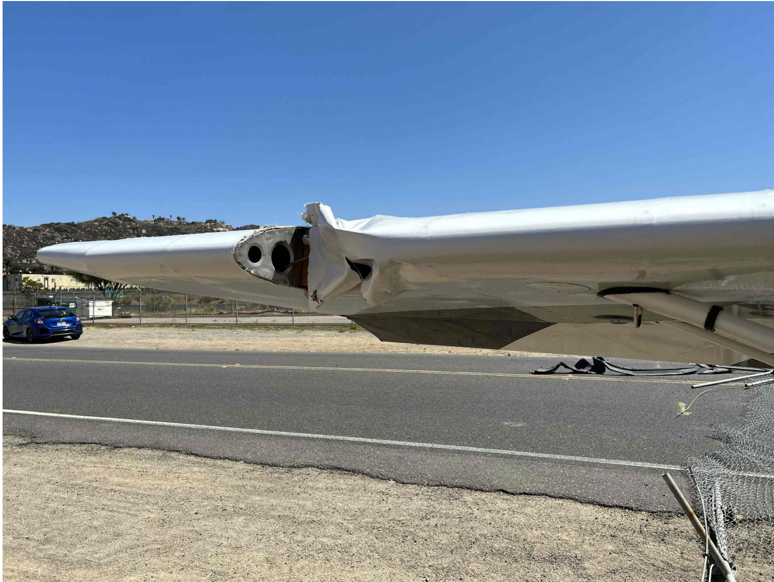
Photograph 2 - Airplane's right wing damage as viewed from the front. (Courtesy of Airport Operations)
