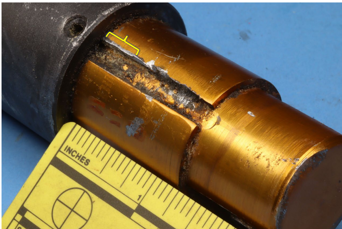
Figure 1. Close views of the lower side of the plunger at the lower forward end of the extension tube. An unlabeled bracket in the upper image indicates contact damage at the right side of the keyway for the plunger consistent with contact with the alignment screw. An unlabeled bracket in the lower image indicates an area where the raised lip at the deformed edge of the keyway was flattened.
