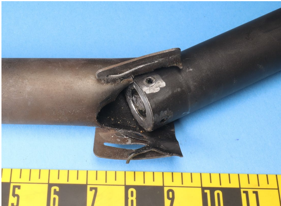
Figure 3. Forward end of the housing showing contact marks and deformation patterns (upper image). In the lower image, the extension tube is shown placed against the deformed surfaces at the forward end of the housing.
