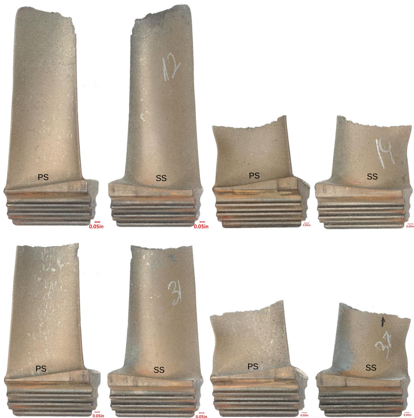
Figure 2 General view of typical blades (#12, #19, #31 and #37) from the set (shown from the pressure and suction sides). Blades #19 and #37 were fractured at approximately 0.595in and 0.630in above the platform respectively. The trailing edge of both these blades was distorted due to impact damage. In contrast, blades #12 and #31 were fractured further up the blade (i.e. approximately 1.769in and 1.302in above the platform respectively) and exhibited limited impact damage apart from small chips/dents on the trailing edges of the blades. All examined blades exhibited limited evidence of necking which suggests no contribution from creep damage lead to the distress.
