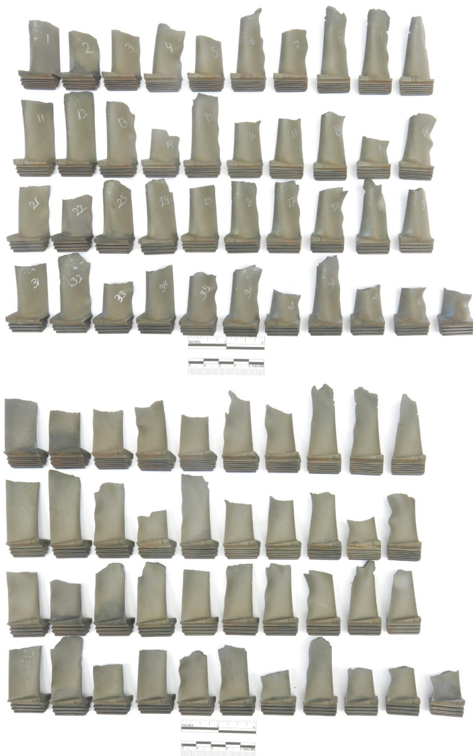
Figure 1 General view of forty-one (41) turbine blades (P/N 3120872-01) viewed from the suction (top) and pressure (bottom) sides, as received for examination. The blades were numbered at disassembly. The blades mostly generally displayed markings associated with heat codes [REDACTED] and [REDACTED] excluding two sets of three blades located diametrically opposite as assembled on the disc (blades #41: [REDACTED], #1: [REDACTED], #2: [REDACTED], #21: [REDACTED], #22: [REDACTED], #23: [REDACTED]). All blades were fractured at various heights and exhibited mechanical damage consistent with impact damage (i.e. most likely domestic object damage or DOD). Limited evidence of necking was observed.
