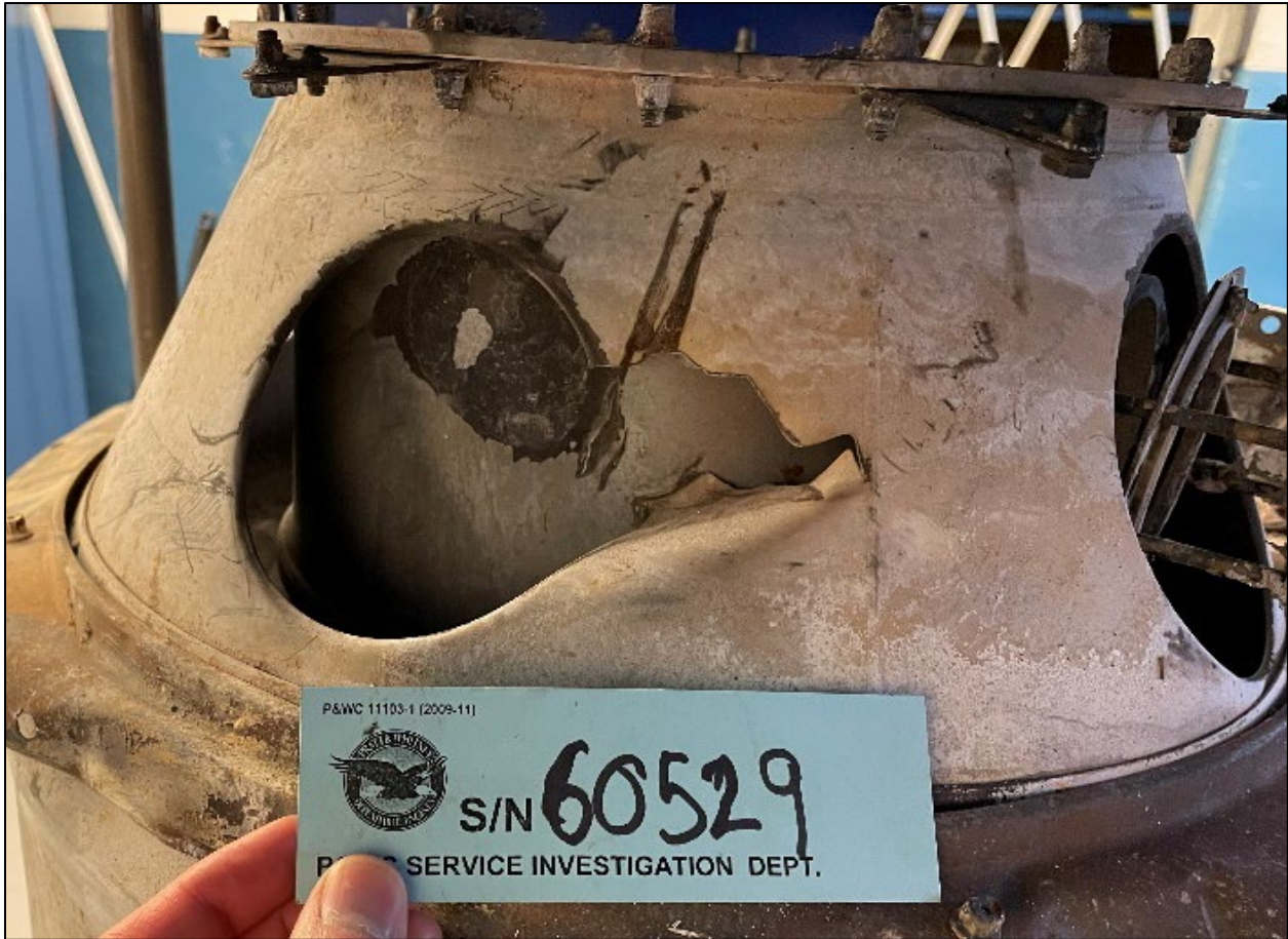
Figure 7. Tear in gas generator case
