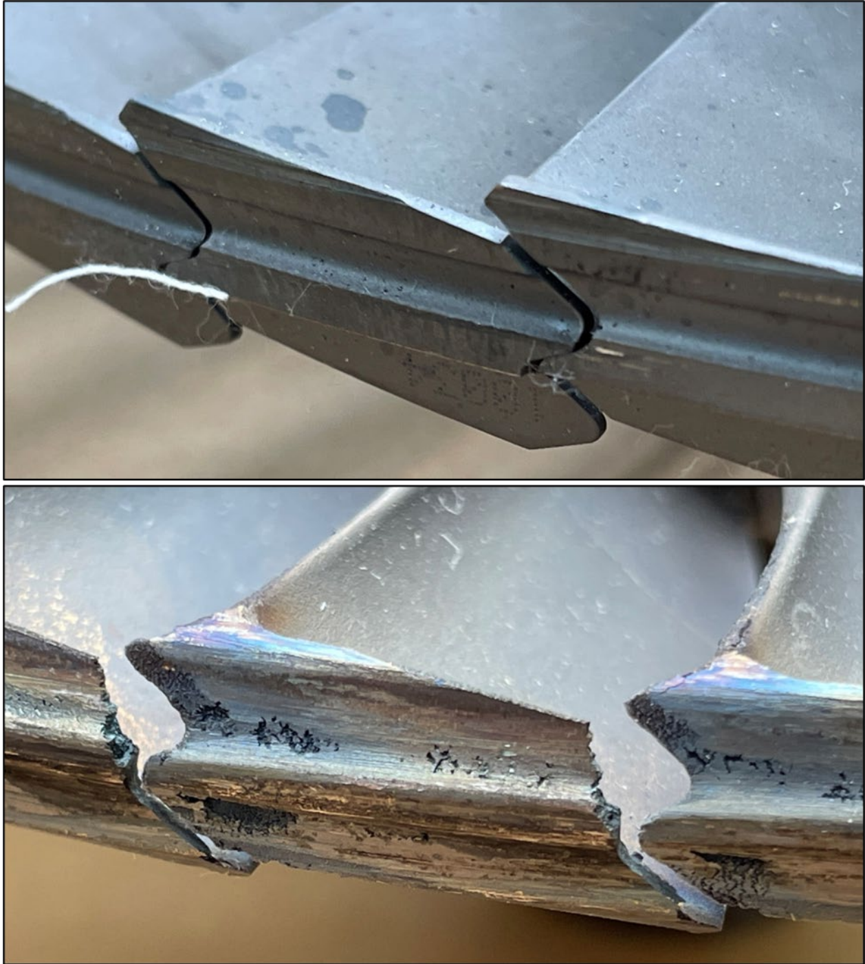
Figure 23. Shroud tips of exemplar PT blades (top) and event blades (bottom)
