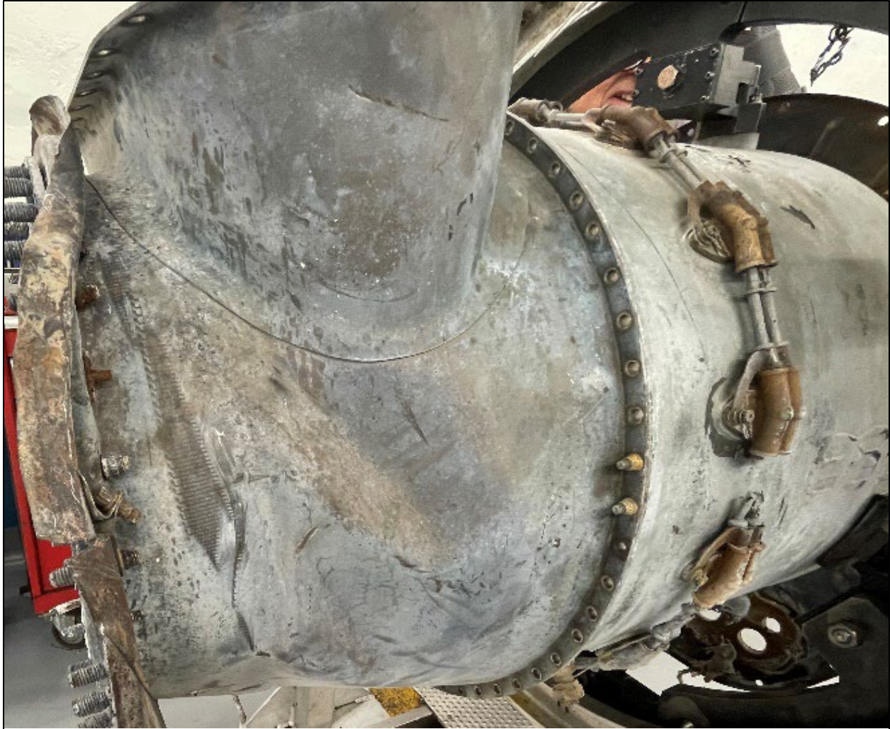
Figure 20. Right engine exhaust case covered with a white coating
