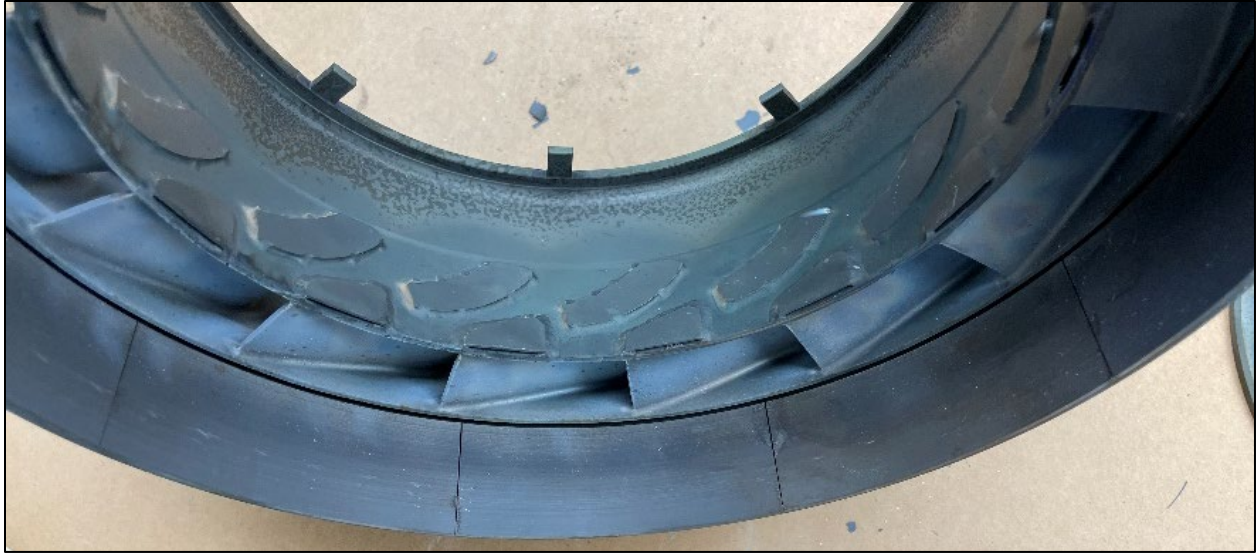
Figure 28. CT vane ring and shroud segments
