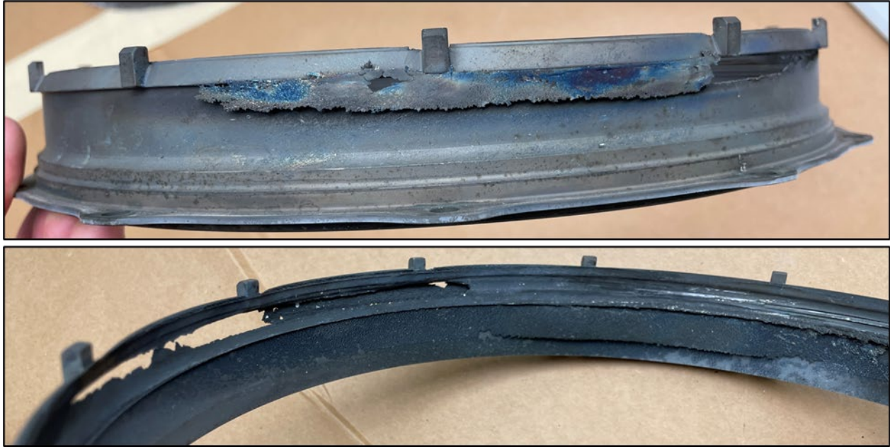
Figure 25. PT outer blade airseal shroud outer (top) and inner (bottom) surfaces
