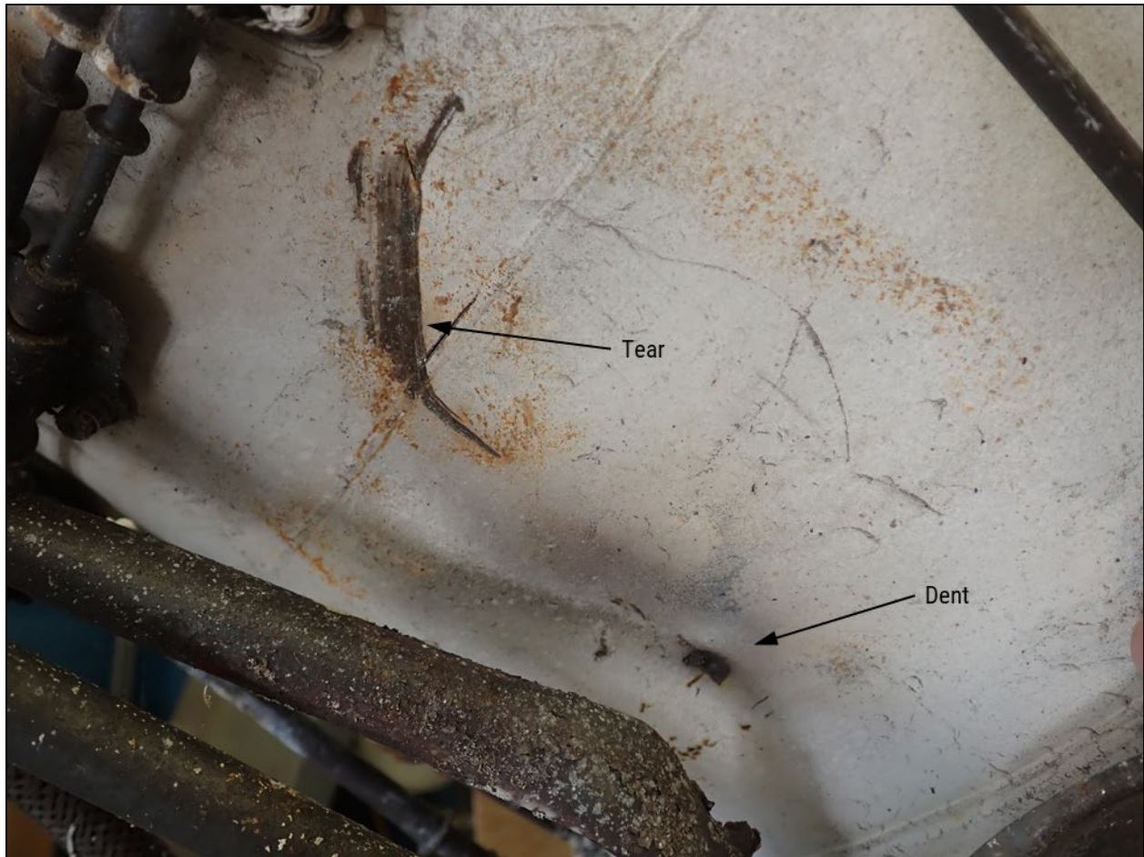
Figure 5. Tear and dent in left engine's gas generator case
