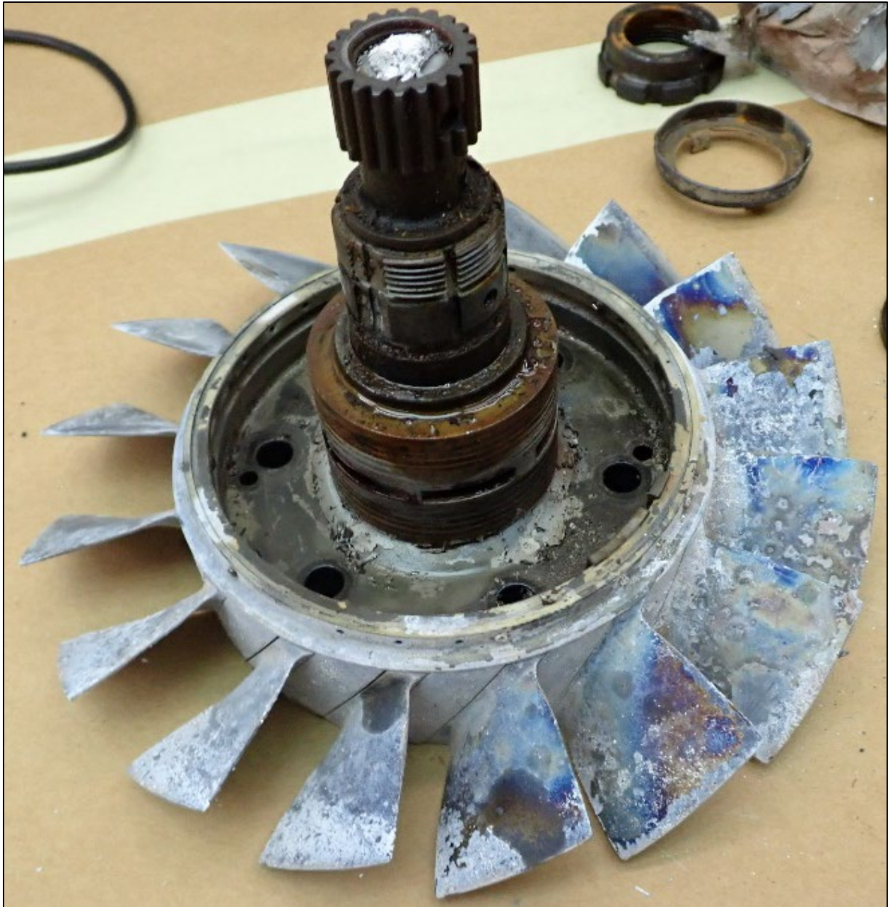
Figure 14. Stage 1 compressor disk assembly covered in white coating
