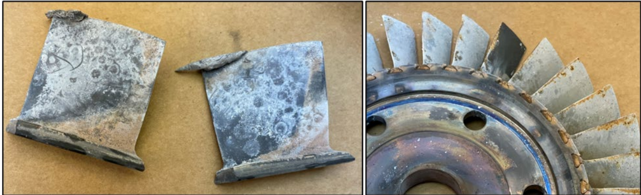
Figure 30. Resolidified metal on stage 1 compressor blade tips (left) and single clean stage 2 compressor airfoil (right)
