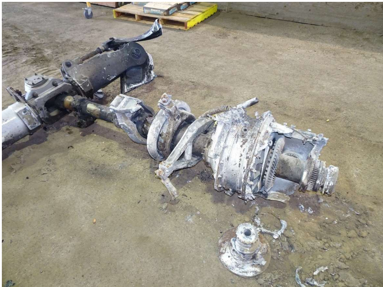
Figure 4. The main transmission was partially consumed by the postcrash fire. The swashplate assembly also exhibited thermal damage.
