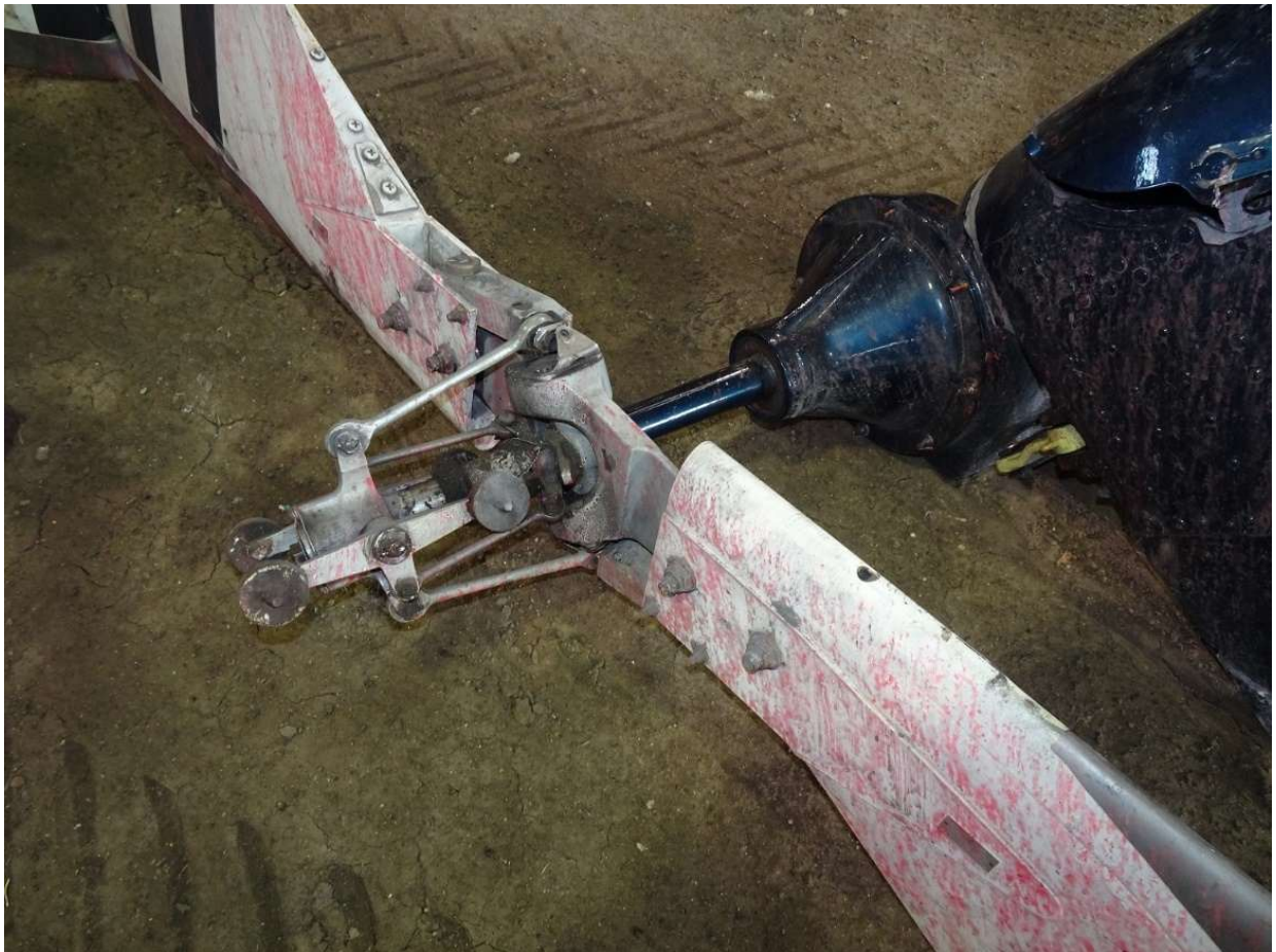
Figure 6. The inboard ends of the two tail rotor blades, the tail rotor head, and the tail rotor gearbox. The red-colored material on the surfaces of the tail rotor is fire retardant that was applied on the wreckage after the accident occurred.
