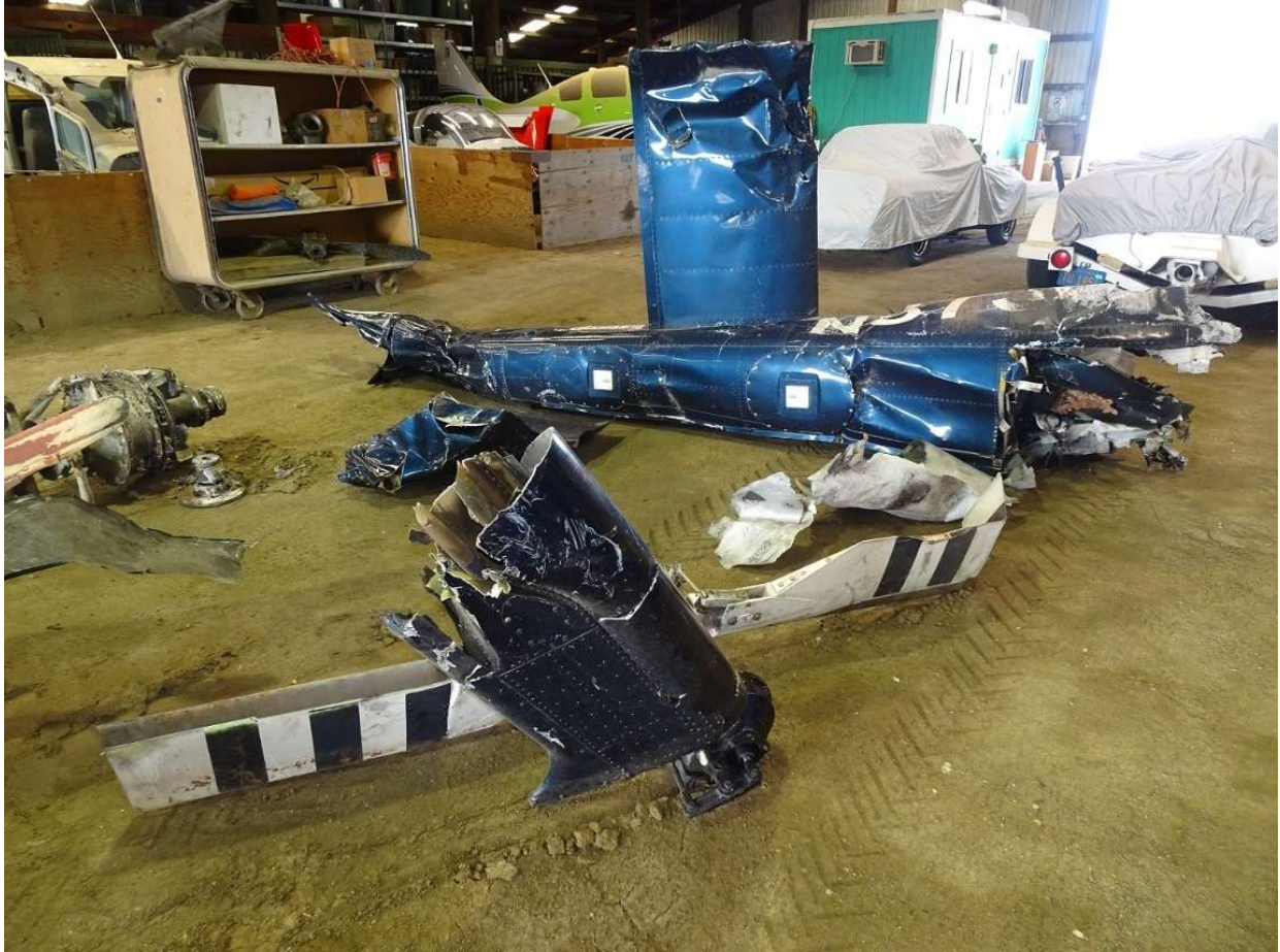
Figure 7. A view of the separated tail boom, with the right horizontal stabilizer attached, and the separated upper portion of the vertical fin with the tail rotor blade spans visible behind it.
