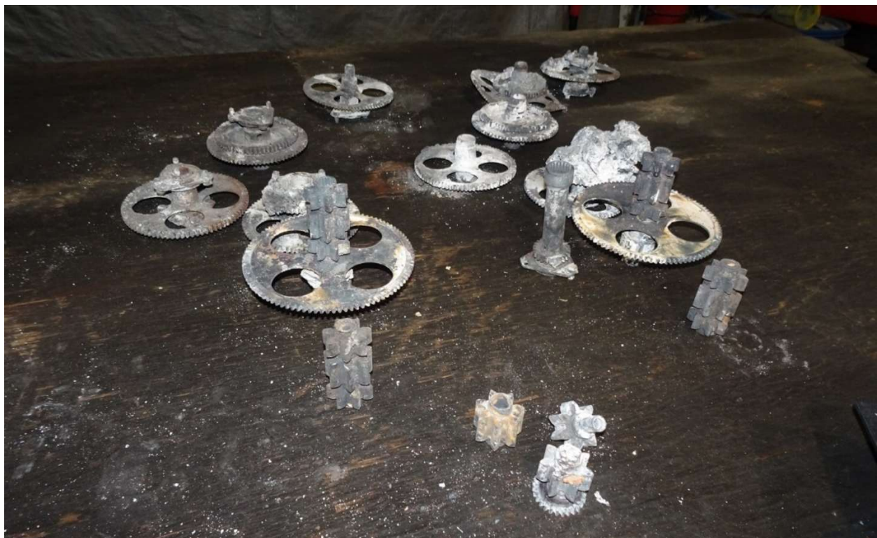
Figure 8. Separated gears found in the recovered wreckage. (The fuel control unit governor flyweight is not shown in this image.)
