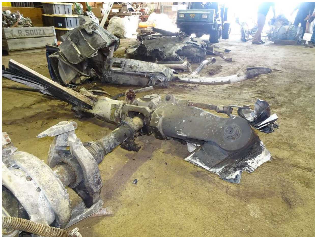
Figure 5. The inboard ends of the main rotor blades, the main rotor hub, and main rotor mast remained as an assembly.
