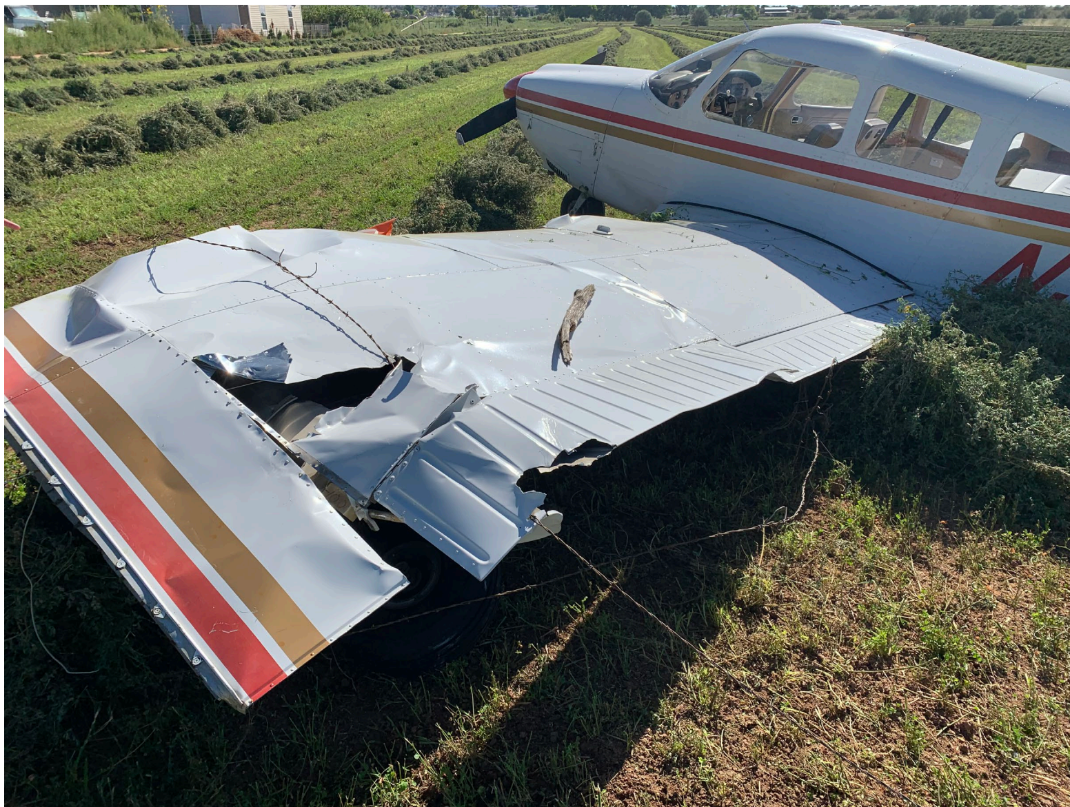
Photograph 2 - View of left wing damage (Courtesy of pilot)
