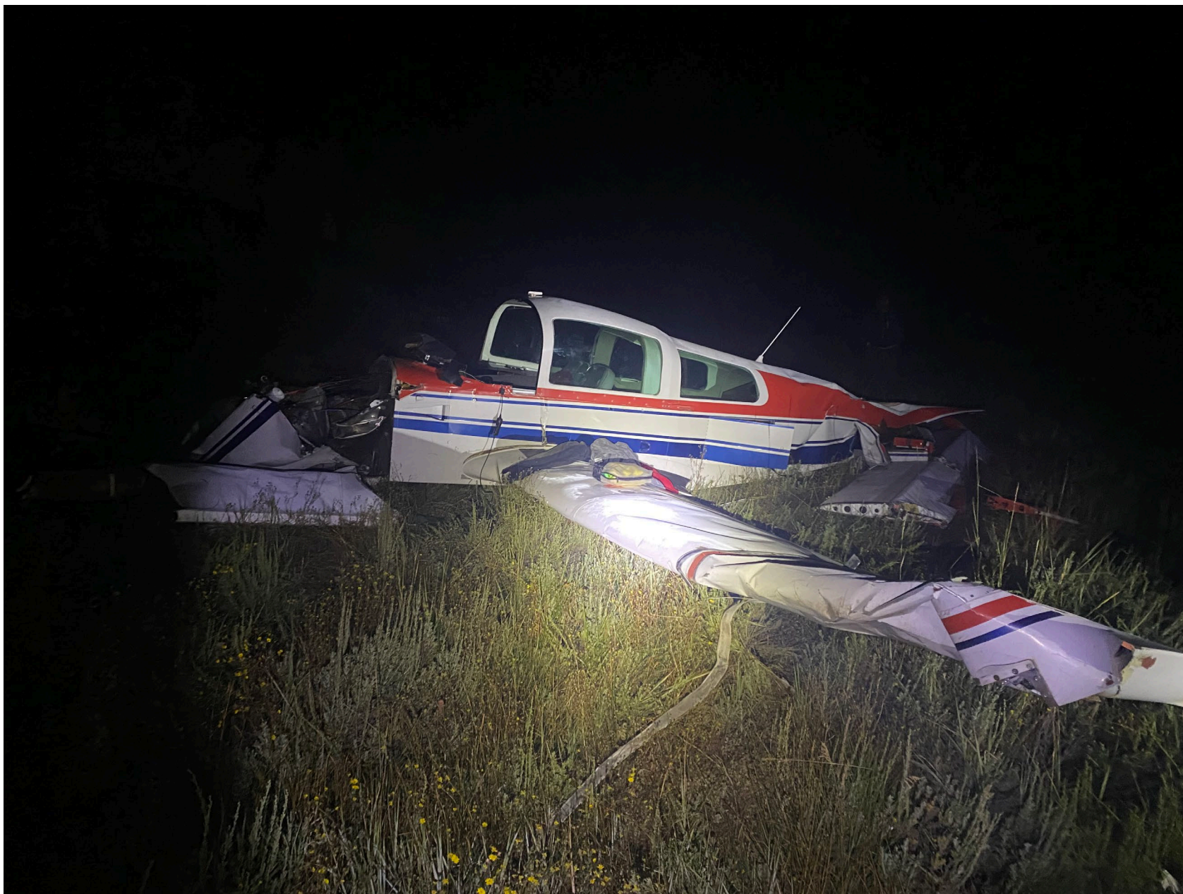
Photo 1 – Left view of airplane with substantial damage to left wing (Photo courtesy of LEO)
