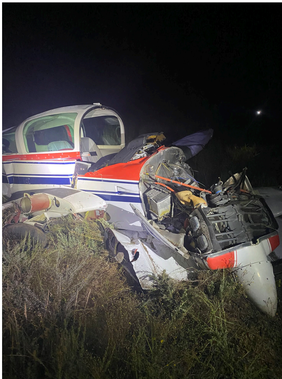
Photo 2 – Front view of airplane with fuselage damage (Photo courtesy of LEO)
