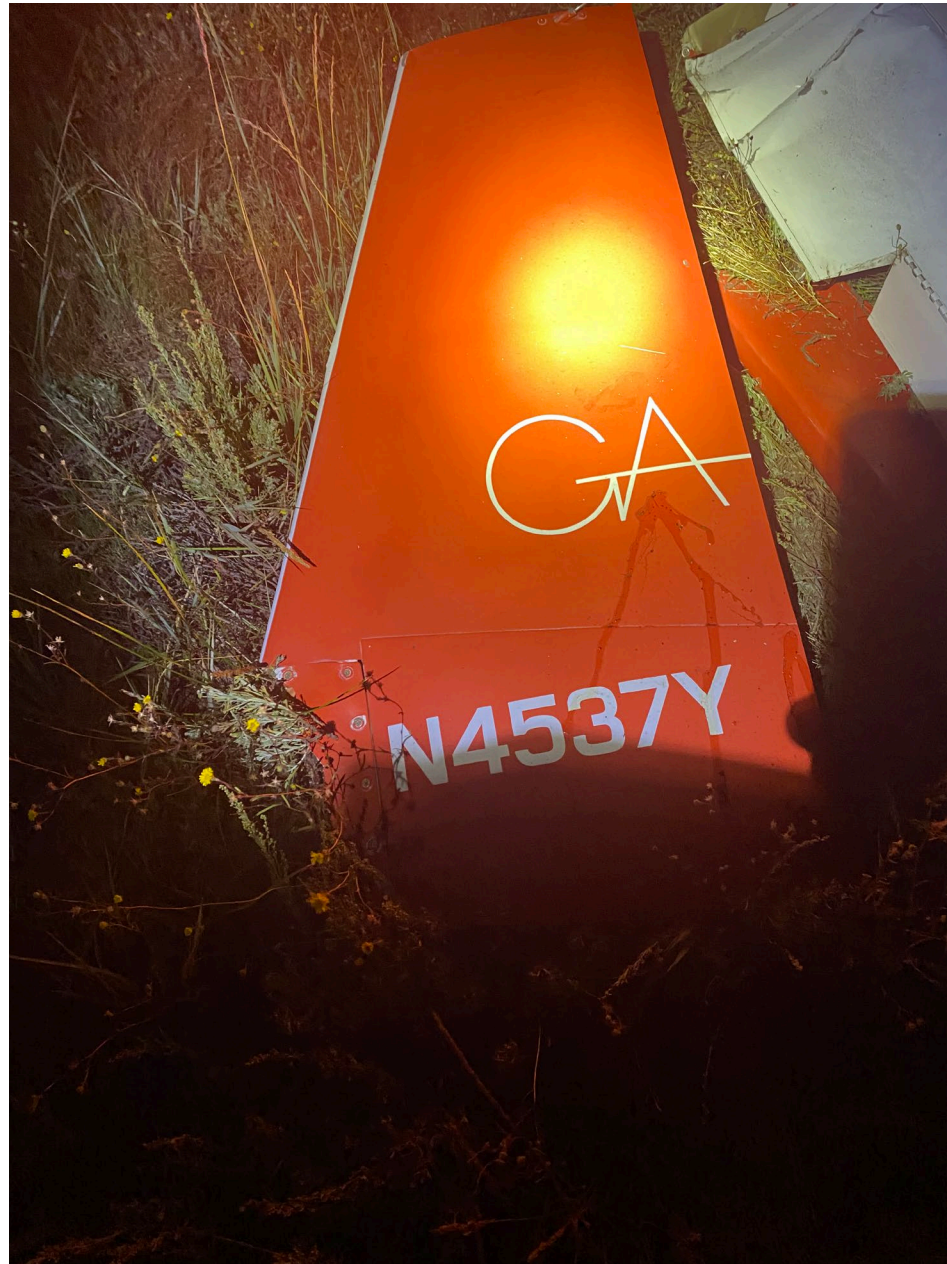
Photo 3 – Rear view of airplane with empennage damage (Photo courtesy of LEO)
