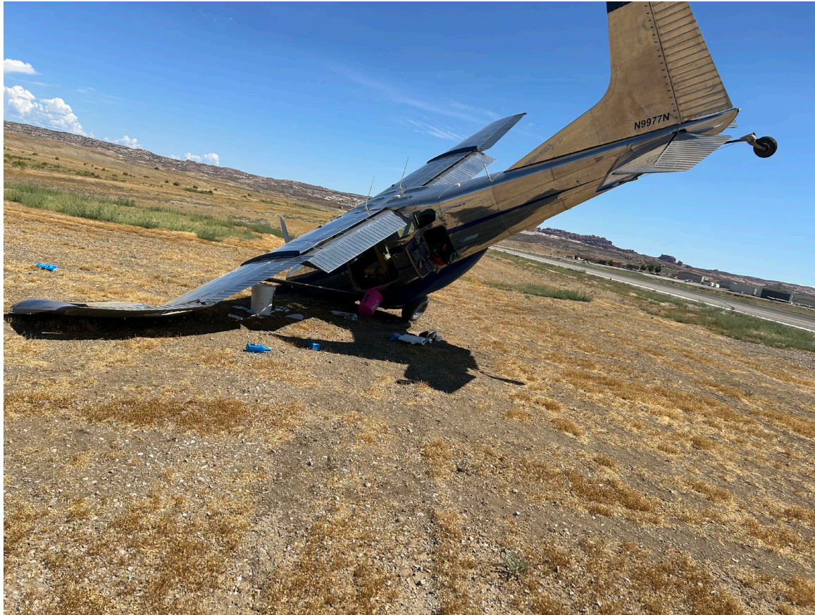
Photograph 1 - View of nosed down airplane with damage to left wing (Courtesy of airport operations)
