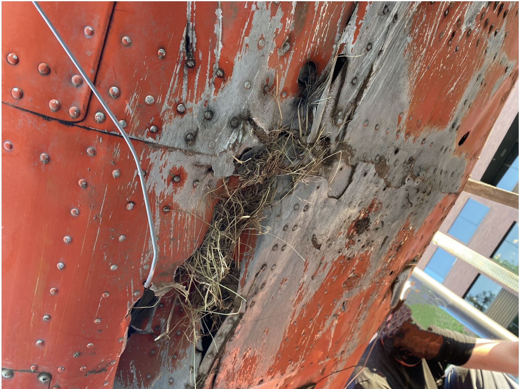
Photo 1 – View of damage on underside of airplane (Photos courtesy of FAA)
