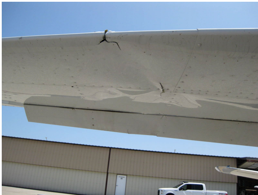
Figure 1 - Damage to right stabilator
