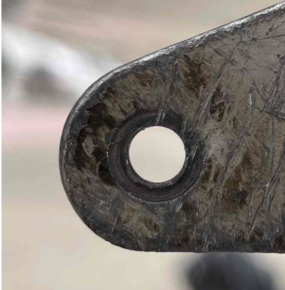
Figure 7 - Circumferential scoring around tab bolt hole.
