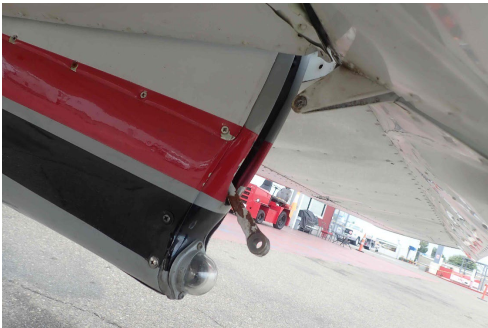
Figure 3 - Stabilator tab actuator disconnected.
