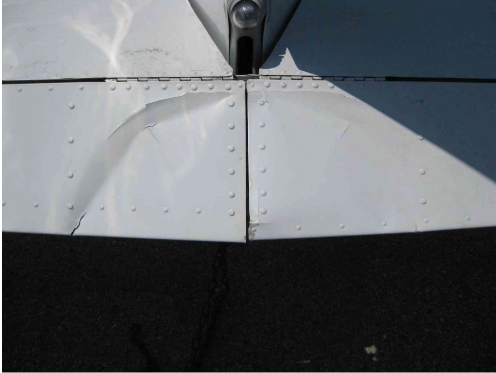
Figure 2 - Stabilator control tab damage.
