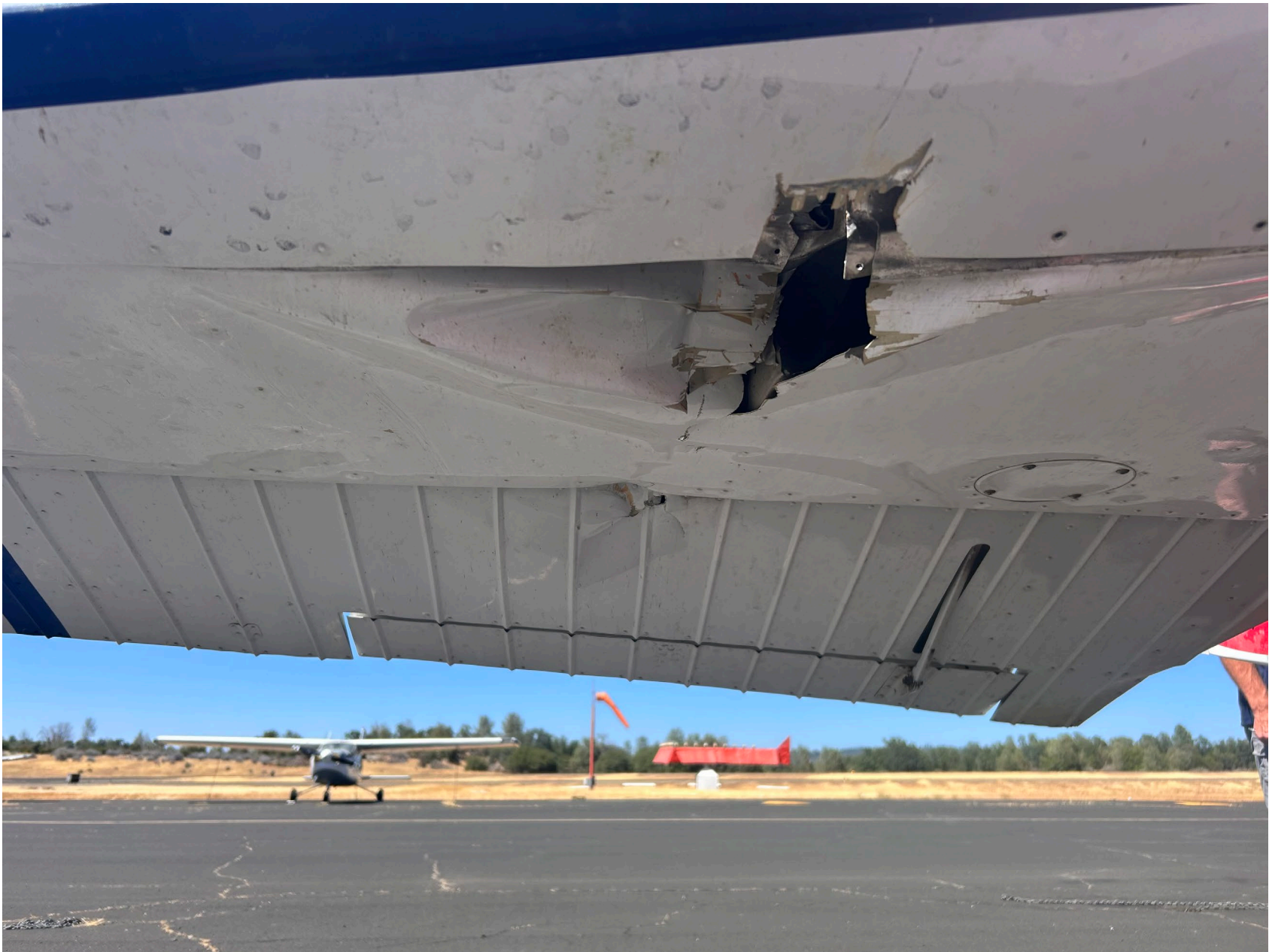
Photo 1 – View of substantial damage to right horizontal stabilizer and elevator (owner)
