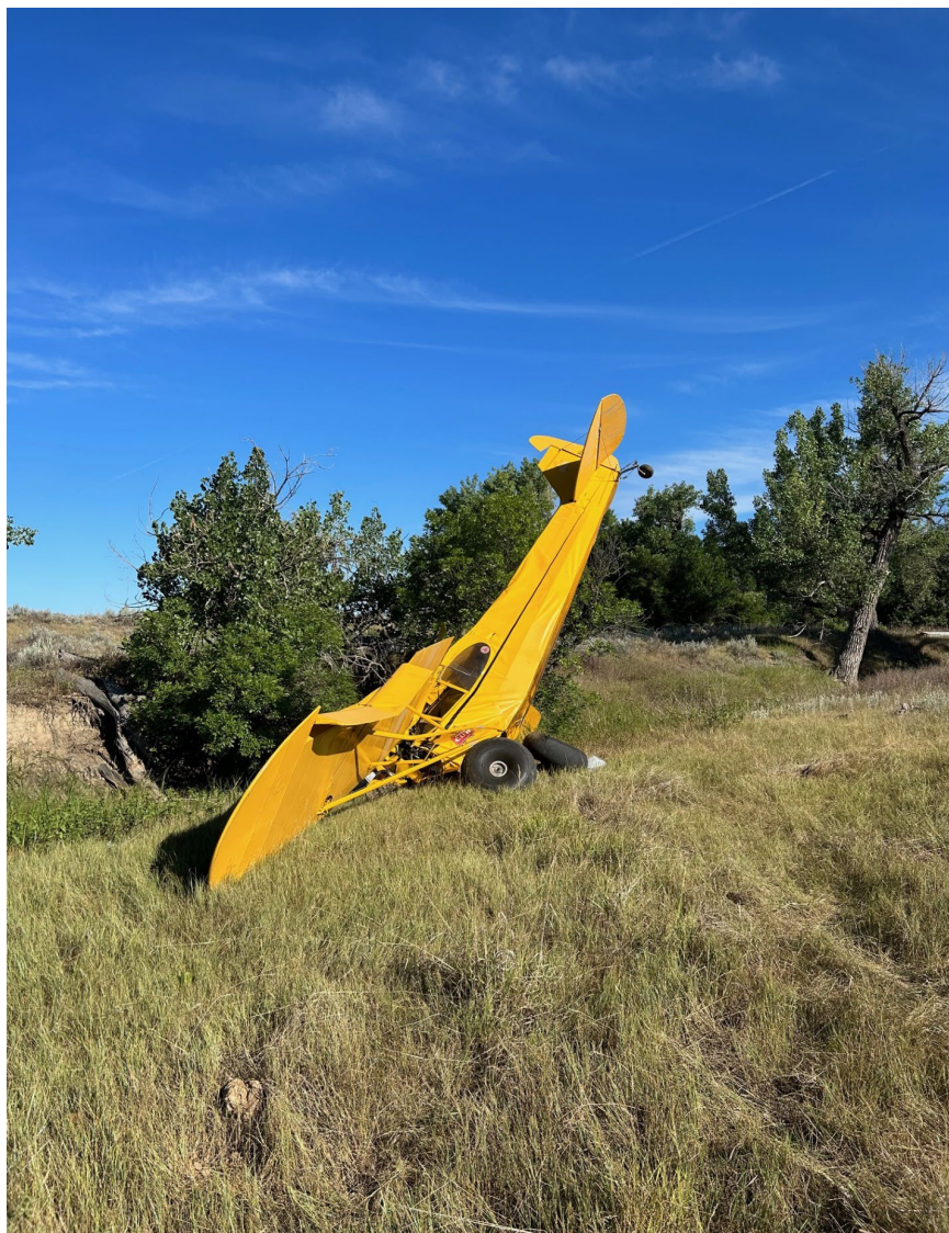
Photograph 1 - View of accident airplane nosed down with damage to left wing (photo courtesy of the local law enforcement officer)
