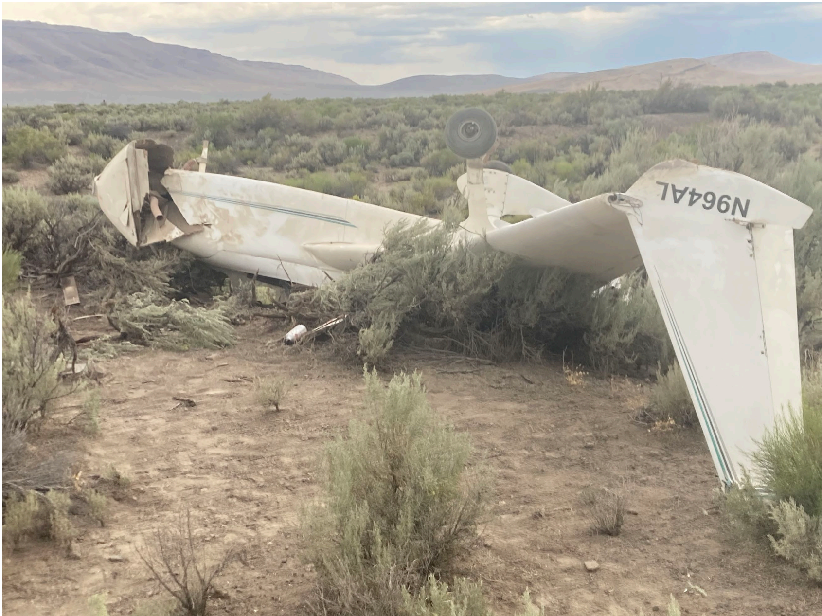
Photo 3 - View of forward fuselage damage (photo courtesy of local law enforcement)
