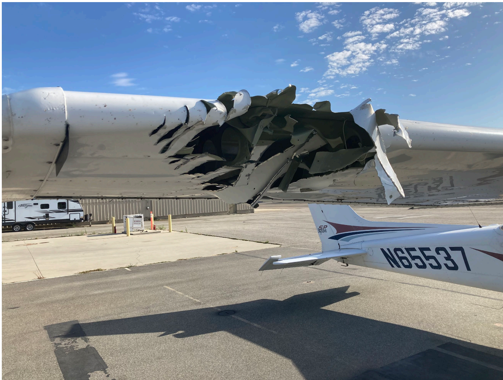
Photo 2 – View of Cessna 172 right-wing damage. (Photos courtesy of operator)
