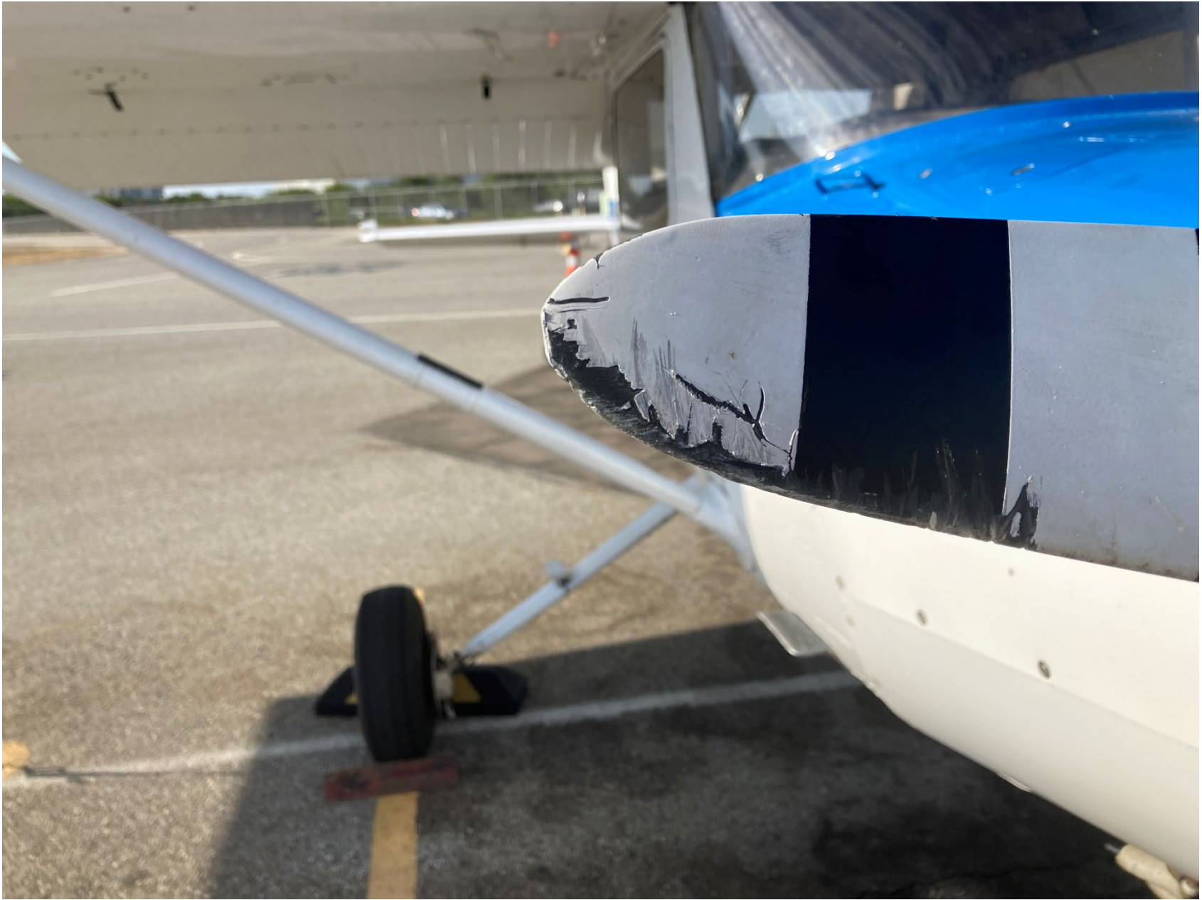
Photo 1 – View of propeller damage of N46393, Cessna 150. (Photo courtesy of operator)
