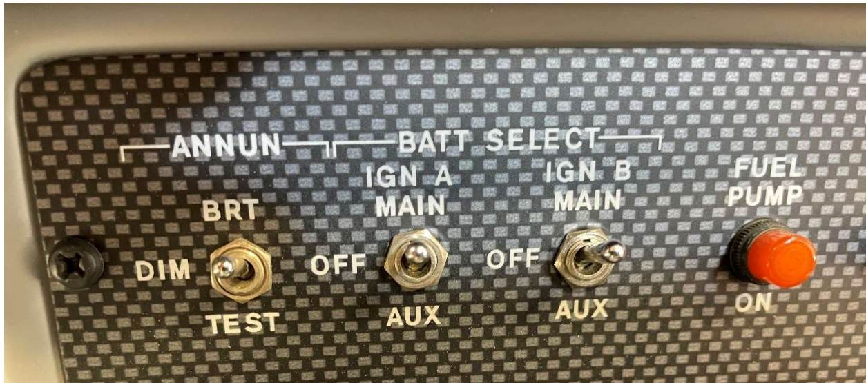
Photograph 2: Battery Switches on Instrument Panel
