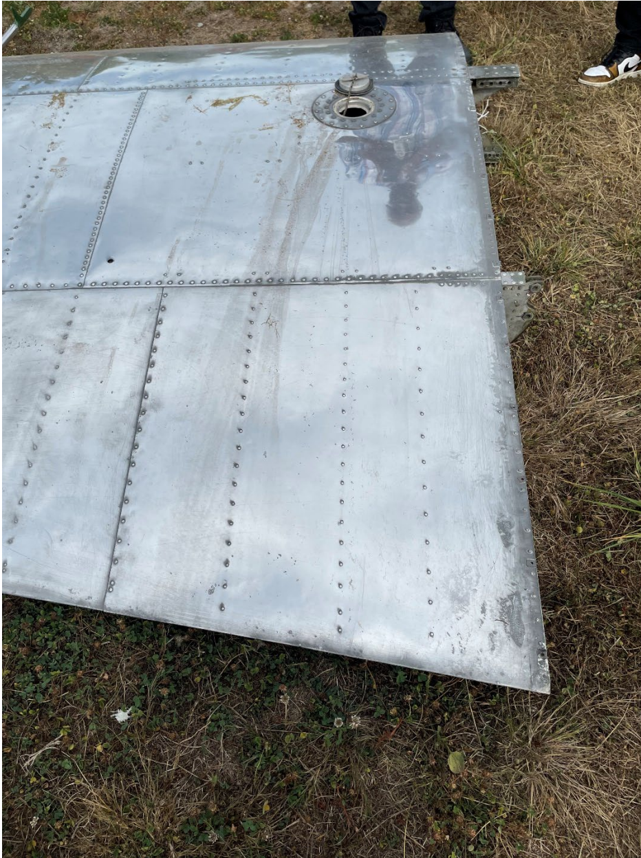
Figure 8. Left-side wing, top view showing the staining that ran aft from the fuel fill port to the end of the wing.
