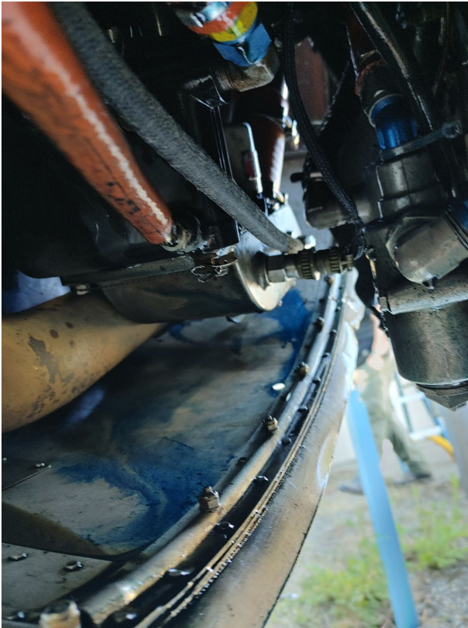
Figure 1. Image of blue staining underneath the carburetor. Image courtesy of the owner.
