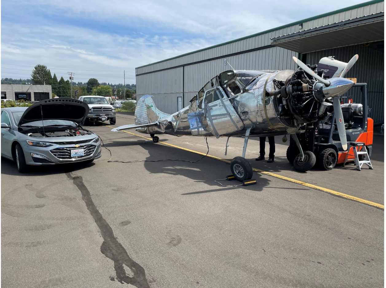
Figure 17. Airplane configured for a test run of the engine.
