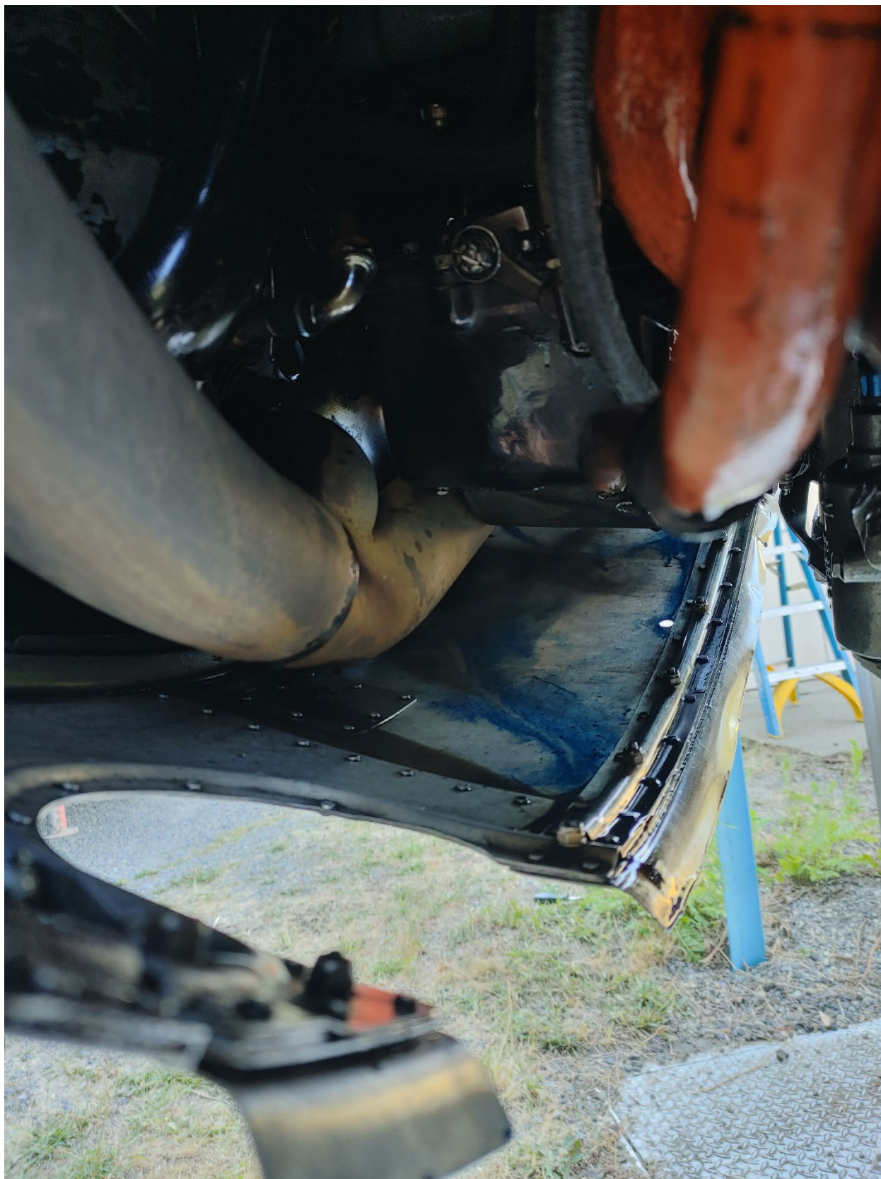
Figure 2. Additional blue staining on cowl. Photo courtesy of the pilot.
