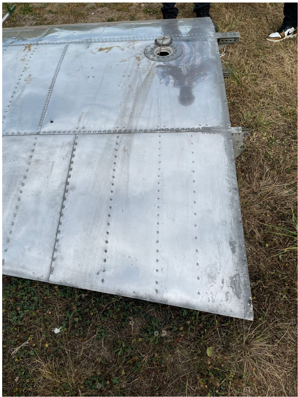
Photo 4 – Left wing showing fuel and dirt stain.
