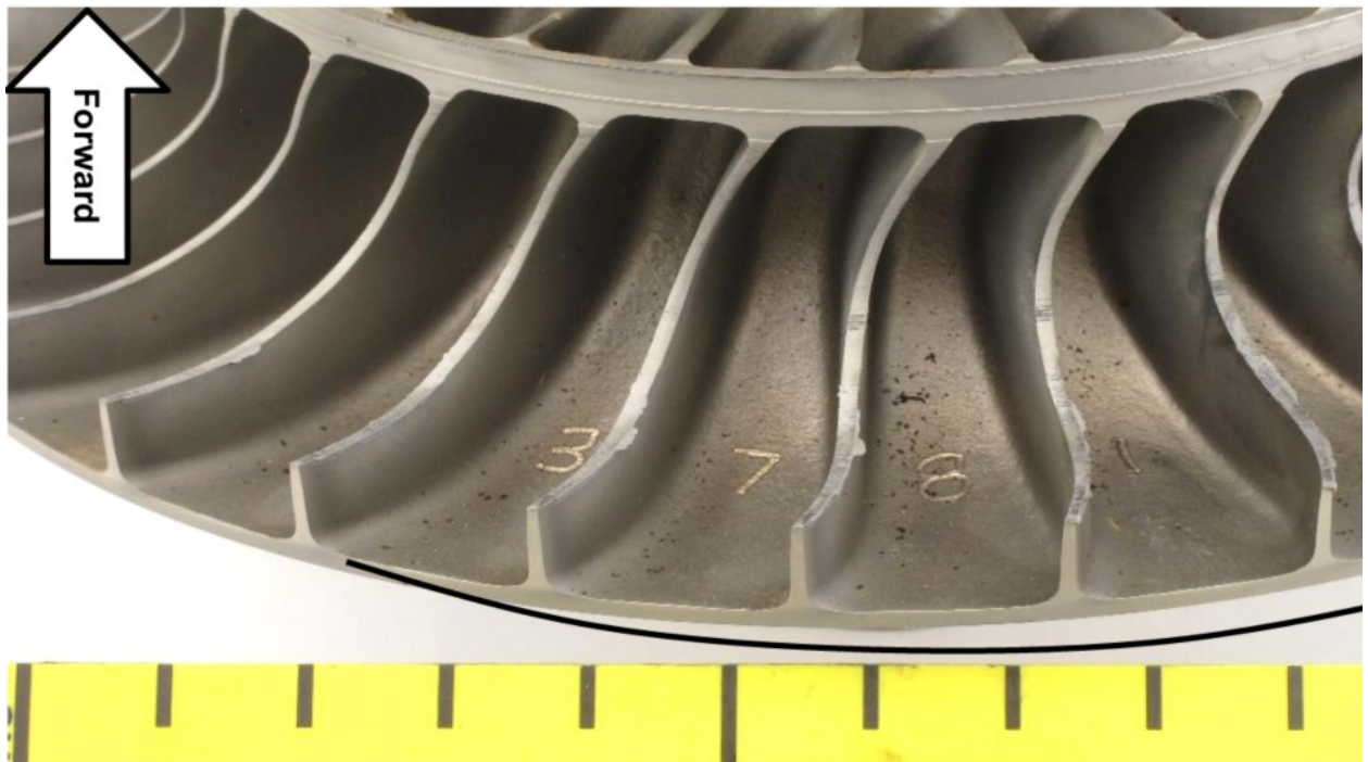
Figure 2. Detailed views of circumferential rub on the compressor impeller.
