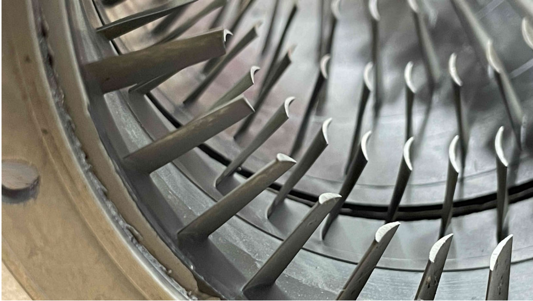
Figure 3 - Rubbing indications from number 5 and 6 blade tips with groove in lining - Engine #2.
