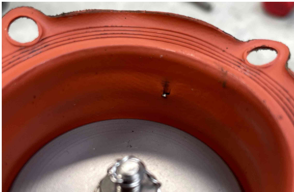
Figure 6 - Hole in diaphragm viewed from the inside - Engine #2.
