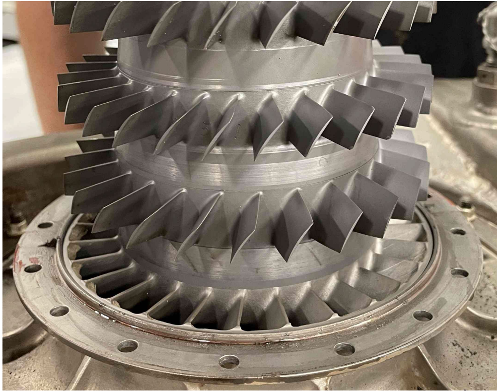
Figure 5 - Compressor blade hub with rub marks - Engine #2.
