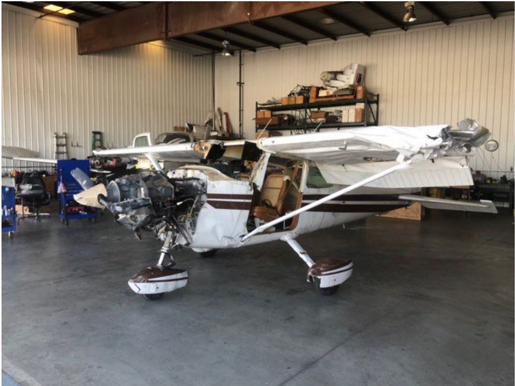
Photo 1 – View of Damage to Wings and Fuselage (Source: Insurance Adjuster)
