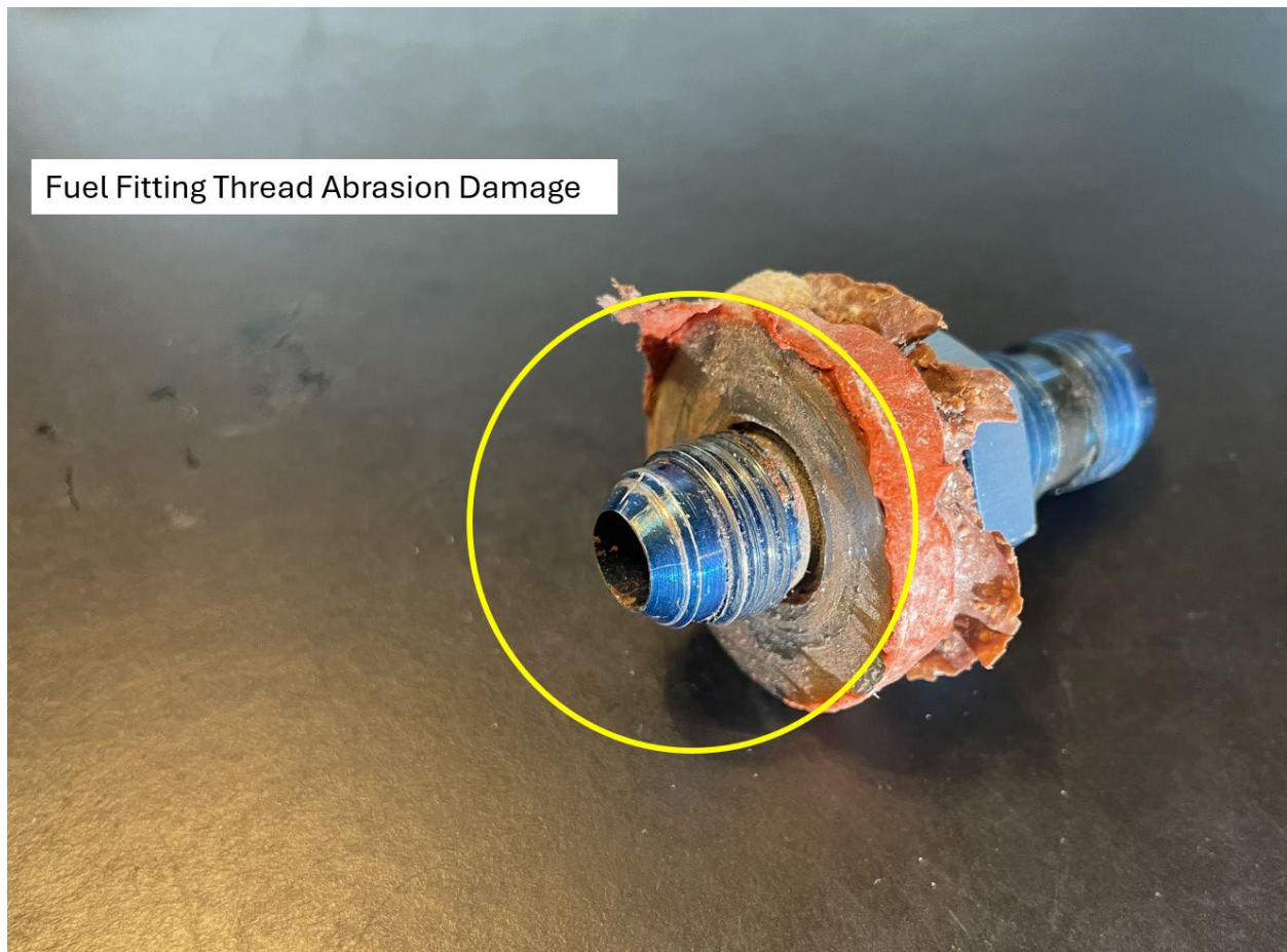
Figure 1 - Fuel Fitting Thread Abrasion Damage
