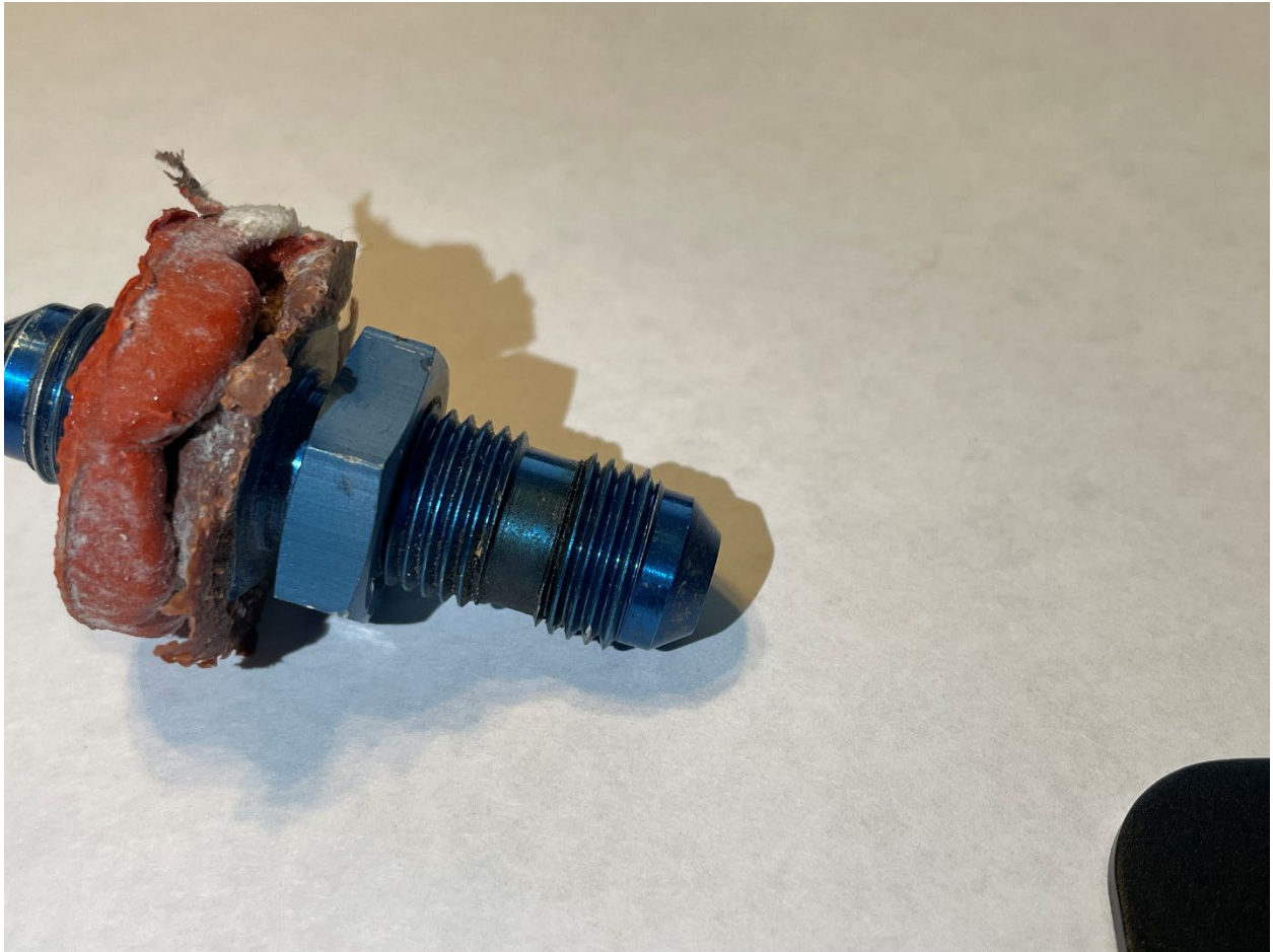
Figure 2 - Undamaged Fuel Fitting Threads
