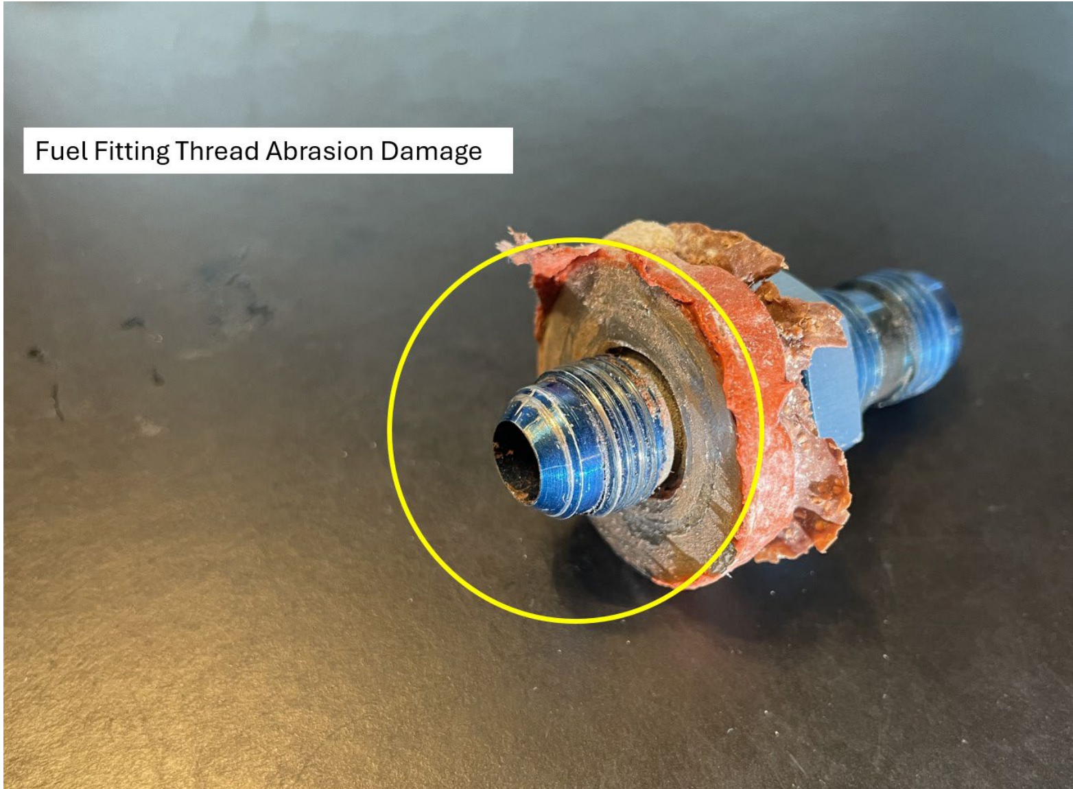
Photograph 3 - Fuel Line Fitting Damage (Courtesy of NTSB)
