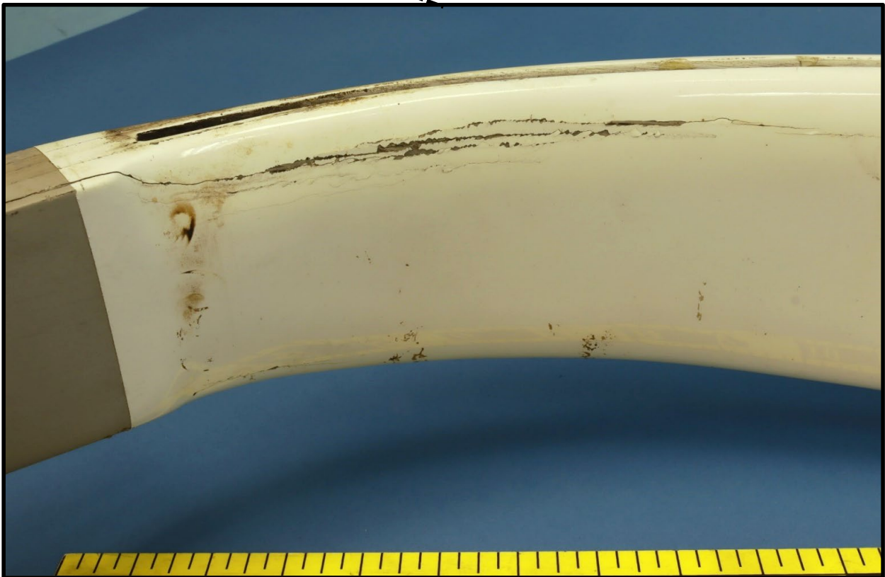
Figure 7. (Top) Overall photo showing the landing gear strut as viewed from the aft side. (Bottom) Close-up photo showing cracks branching onto the inner surface of the strut on the left side.
