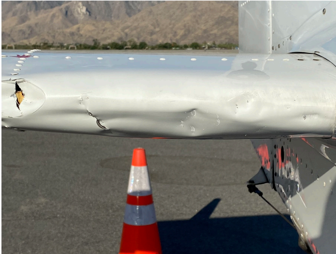
Photograph 3 - Horizontal stabilizer damage
