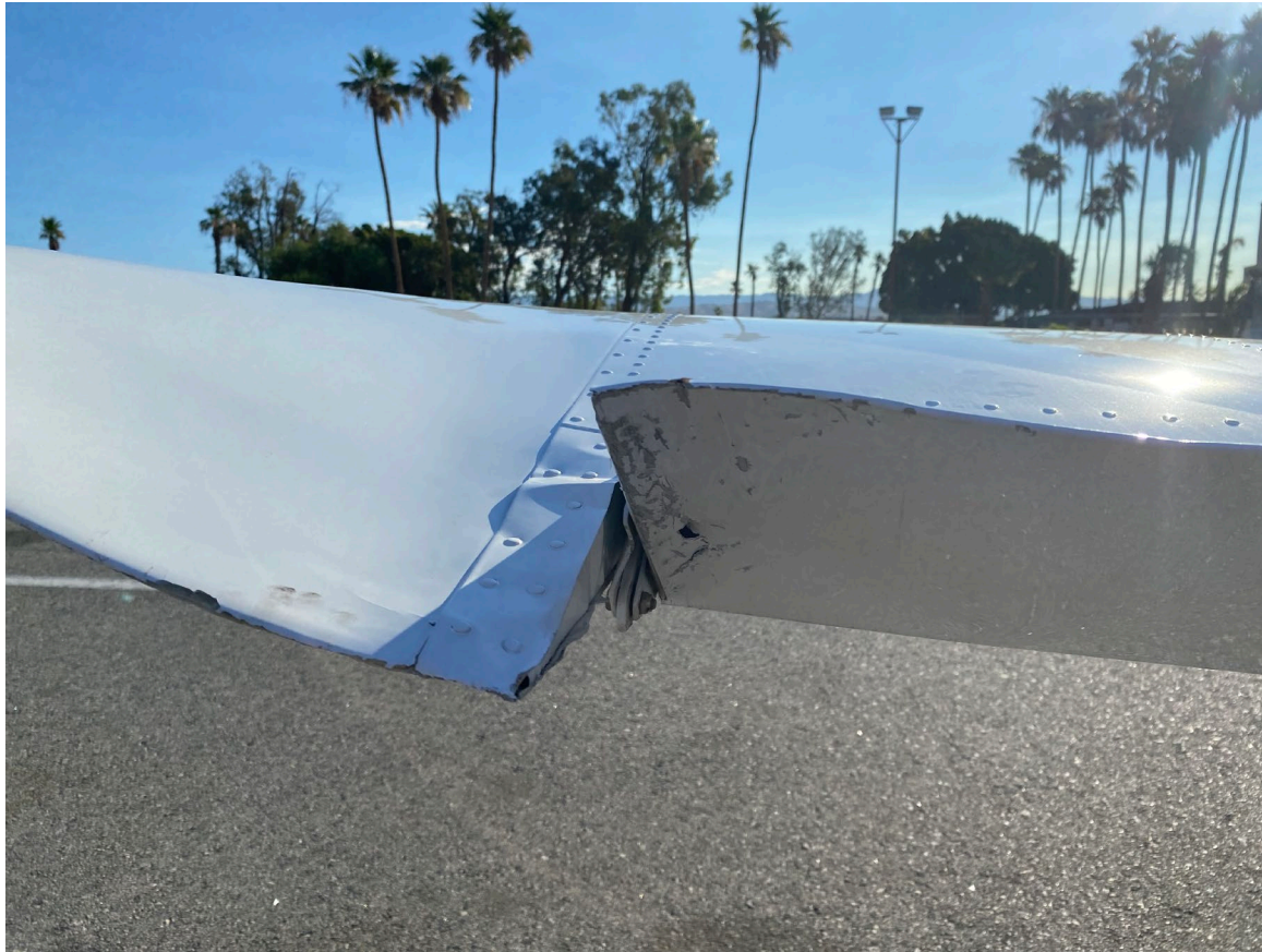
Photograph 2 -Left wing damage
