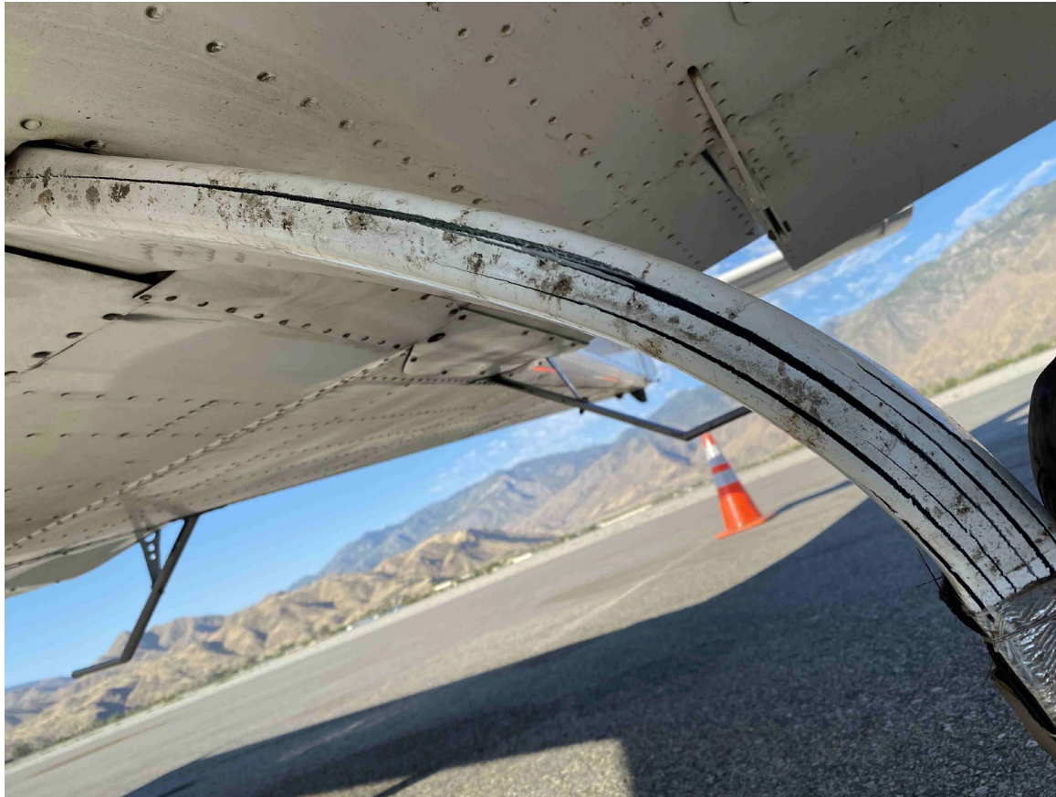
Photograph 1 - Left leg damage
