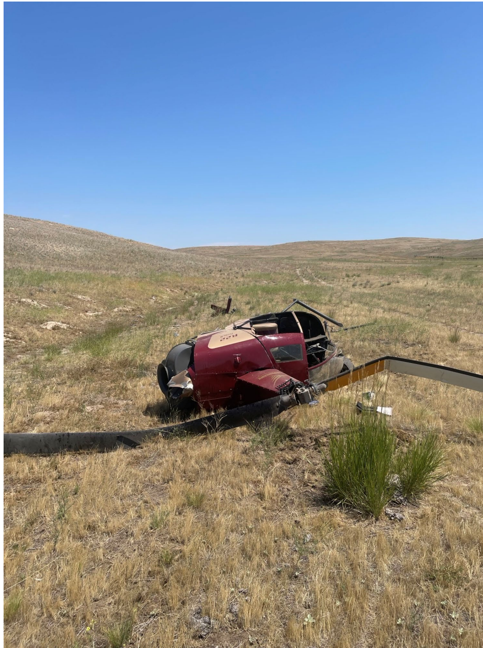
Photo 1 – view of damage to tailboom and tail rotor assembly (pilot)
