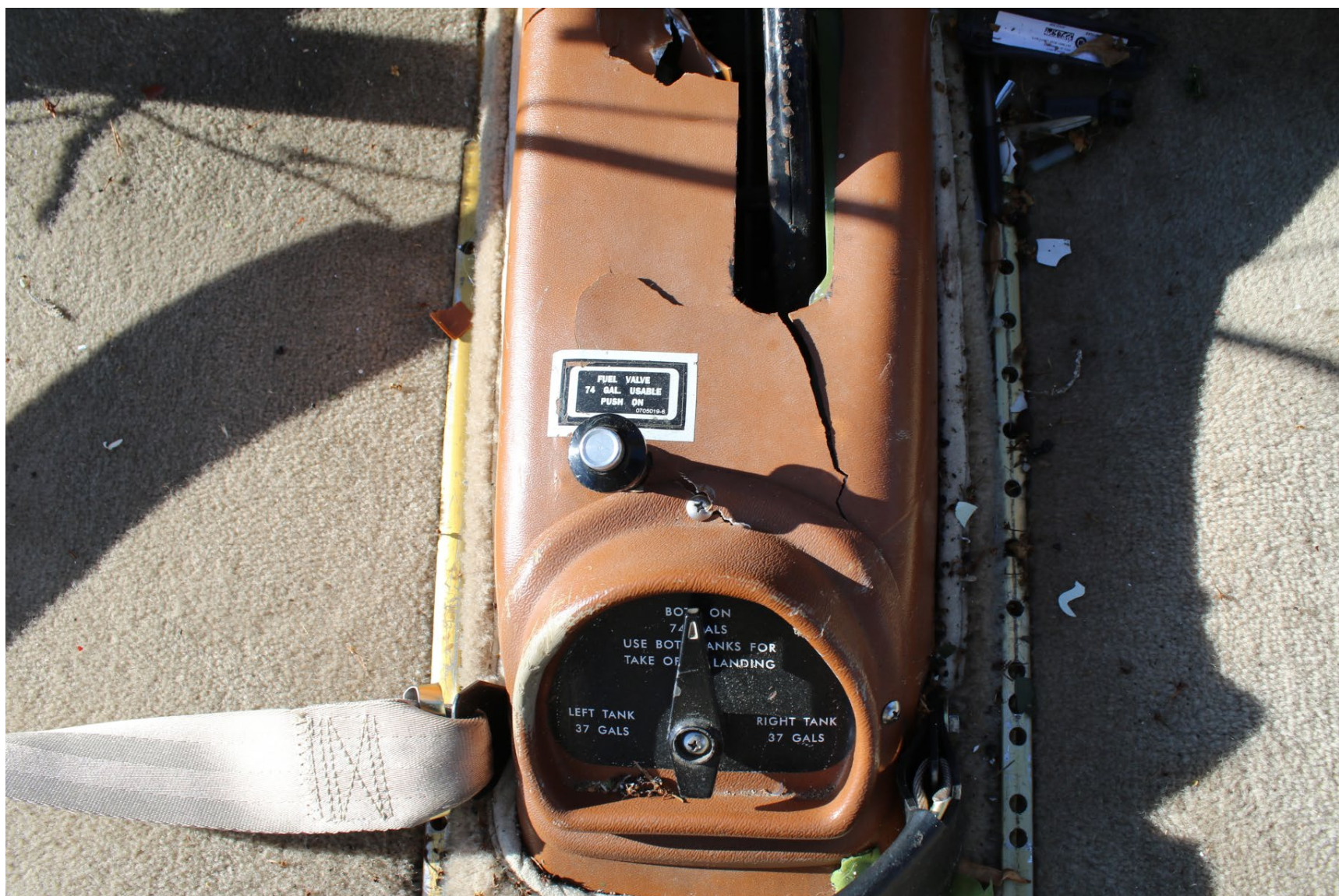
Photograph 2 - View of fuel selector valve lever position set to BOTH ON at accident site (Courtesy of FAA)
