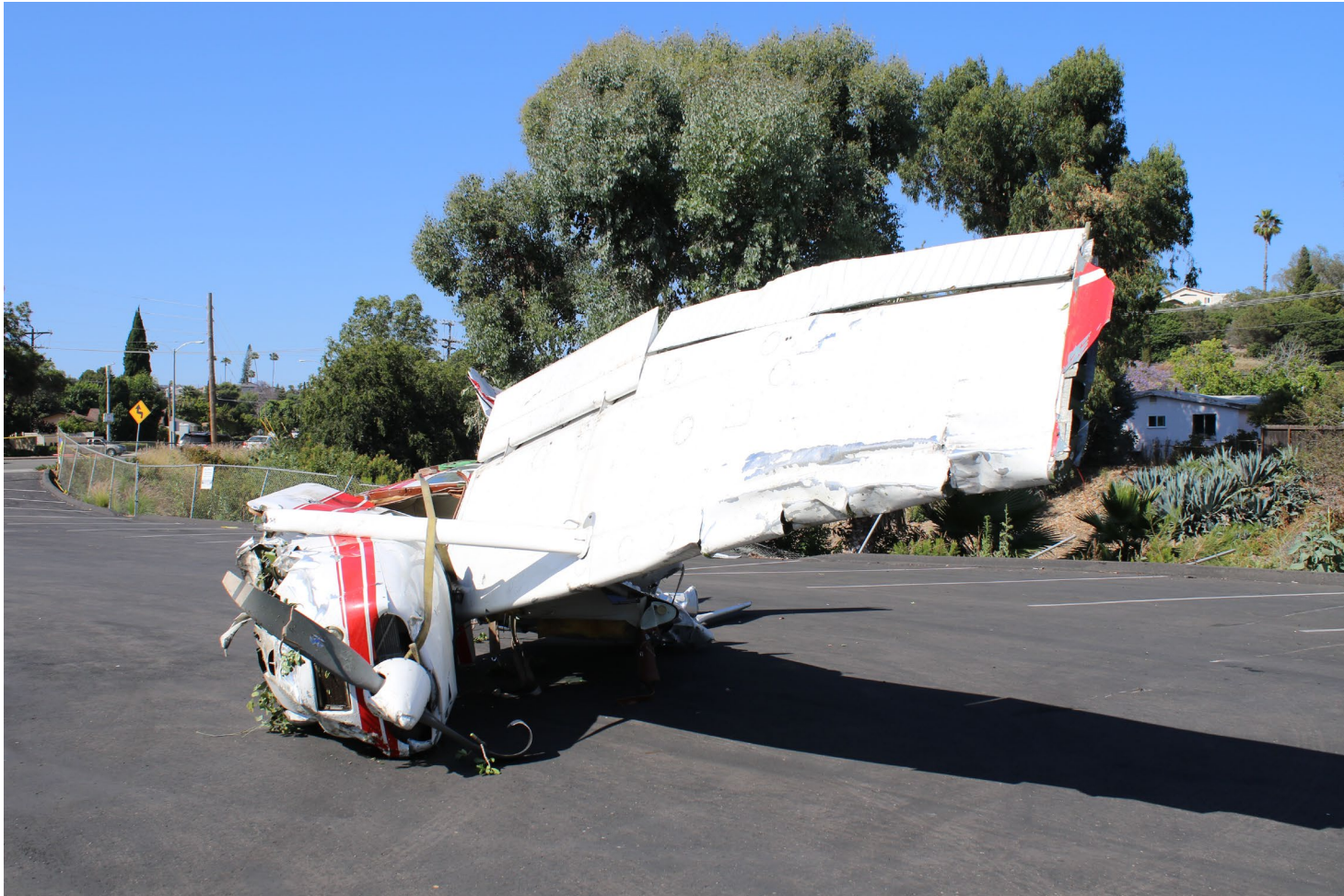
Photograph 1 - View of recovered accident airplane with damage to right wing and fuselage (Courtesy of FAA)
