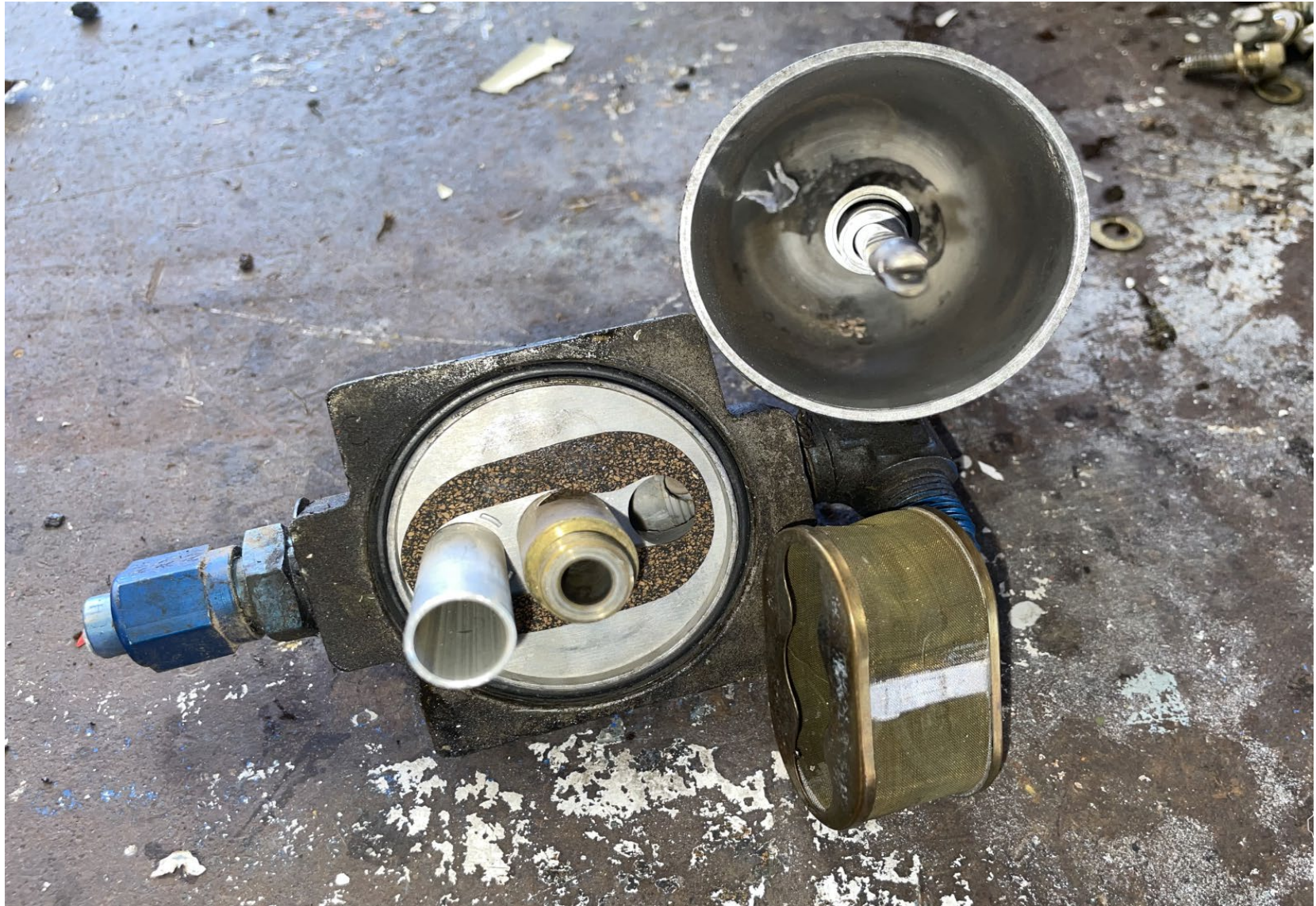
Photograph 7 - View of removed damaged fuel filter bowl
