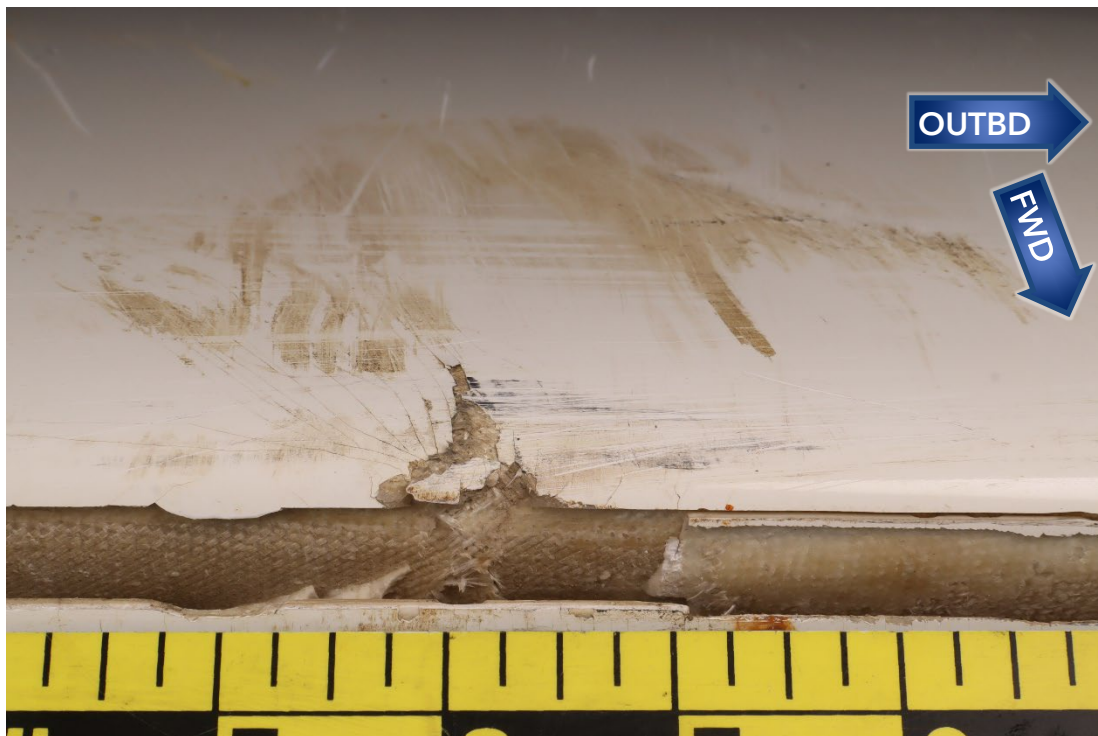
Figure 5. Leading edge impact damage on the lower skin with black and brown deposits on the adjacent surfaces.
