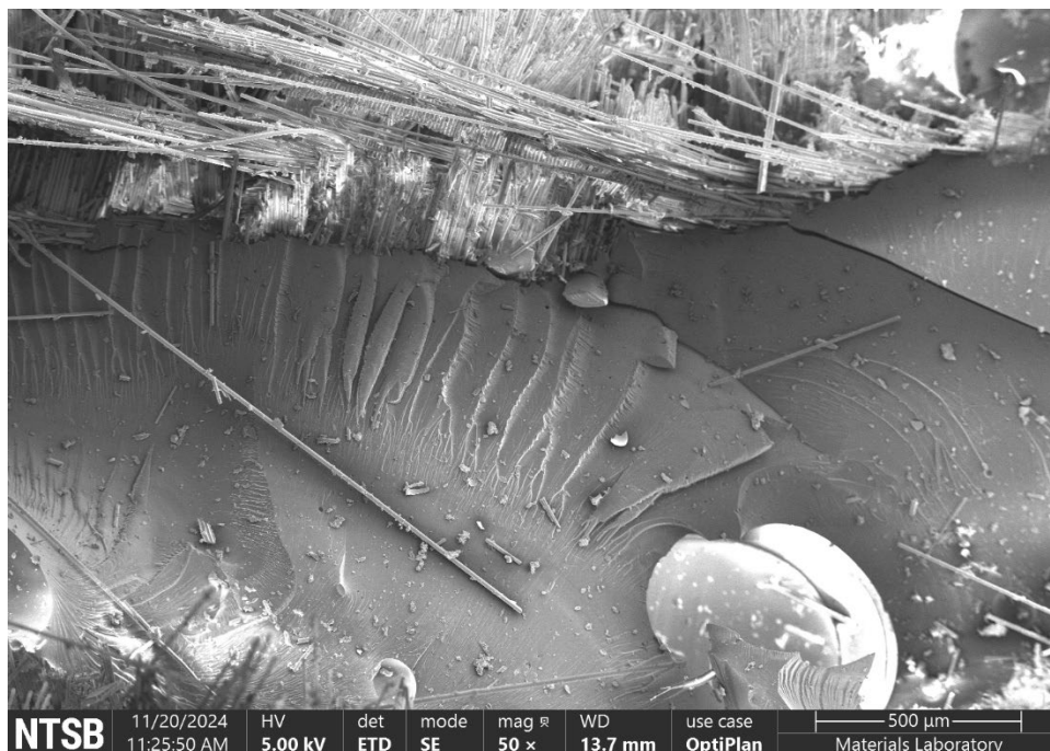
Figure 19. SEM image of a resin rich area above the wrinkle forward of the resin pocket on the outboard side of the fracture through the right wing spar lower cap.
