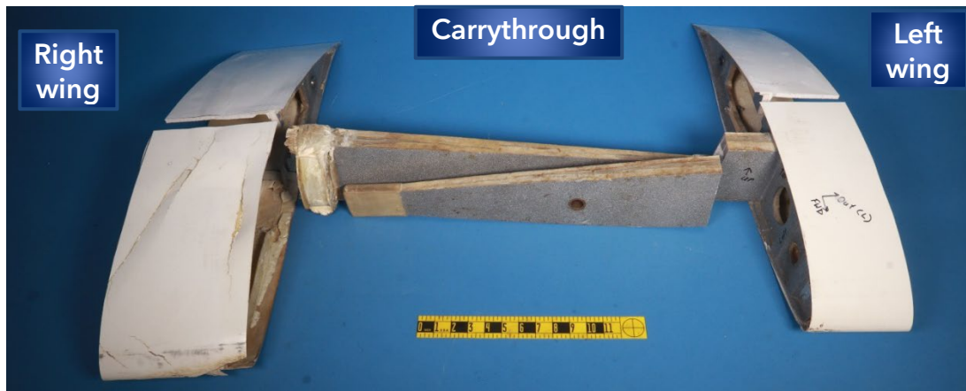
Figure 10. Right and left wing pieces and carrythrough beams after sectioning.
