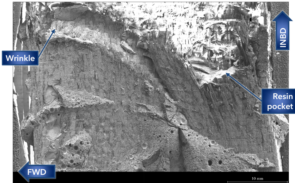
Figure 20. Montage of SEM images stitched together to show fracture features at the lower surface of the right wing spar lower cap outboard of the fracture.
