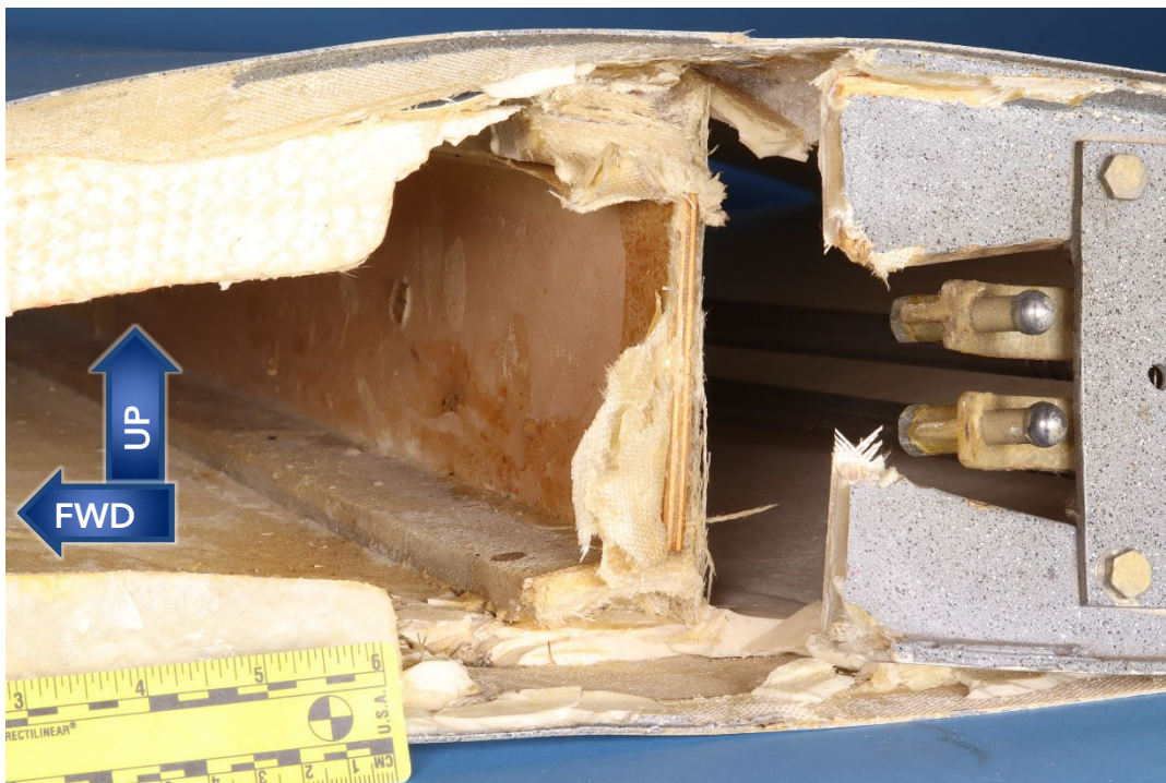
Figure 9. Outboard side of the right wing spar fracture at the inboard end of the wing.
