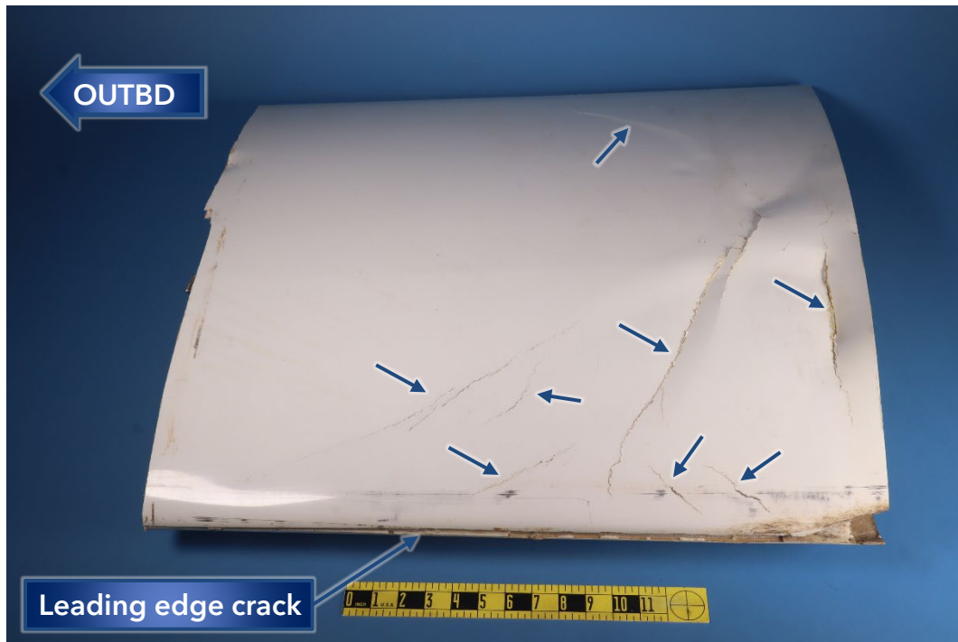
Figure 2. Upper surface of the right wing piece.
