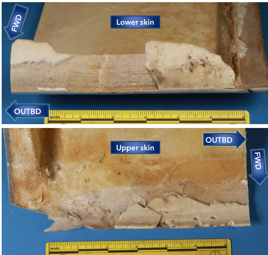
Figure 11. Sectioned right wing lower skin (upper image) and upper skin (lower image) after the upper skin was separated from the spar and lower skin showing mating fracture surfaces at the inboard end of the leading edge bond line.
