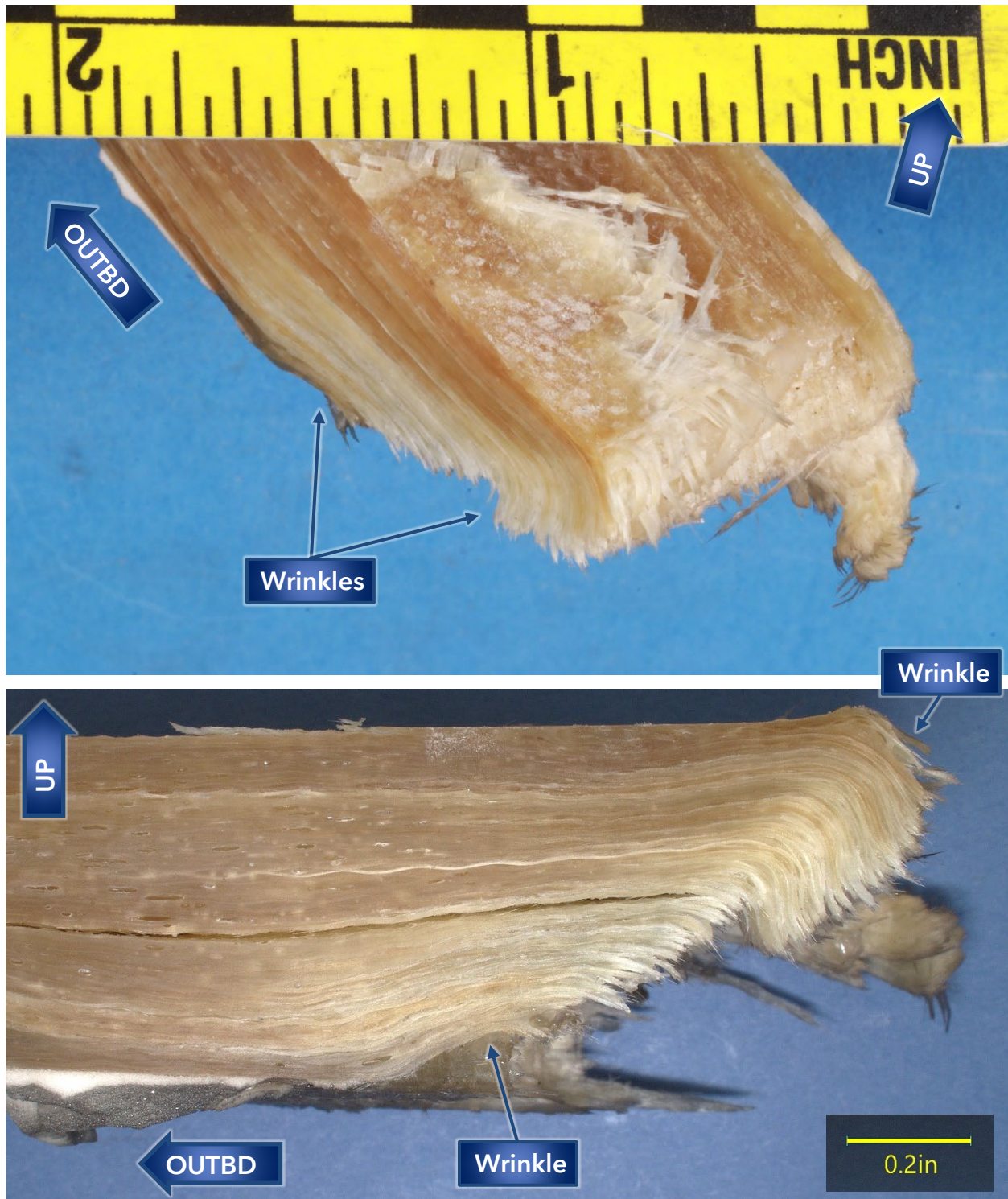
Figure 22. Spanwise cross-section through the right wing spar lower cap piece showing composite layers outboard of the fracture surface.
