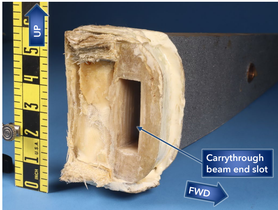
Figure 8. Inboard side of the right wing spar fracture at the outboard end of the carrythrough beam.
