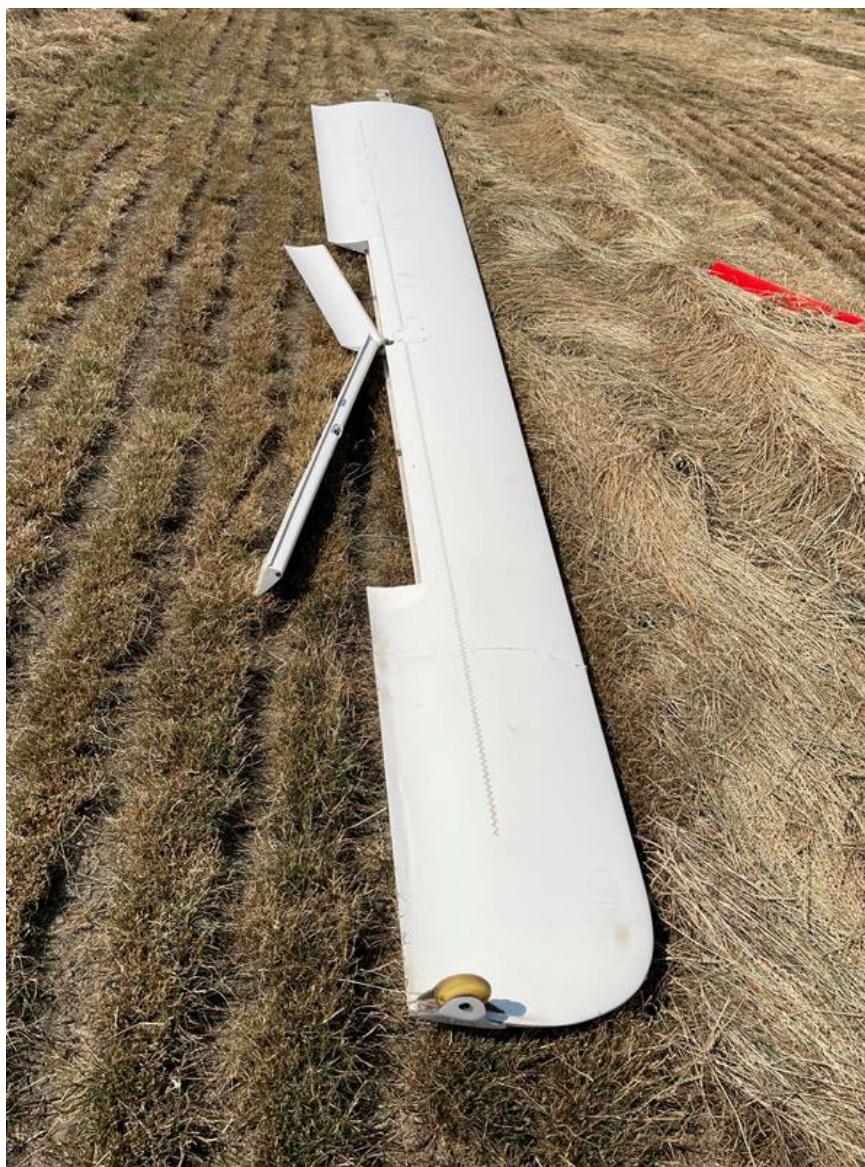
Photograph 2 - View of separated left wing (Courtesy of FAA)
