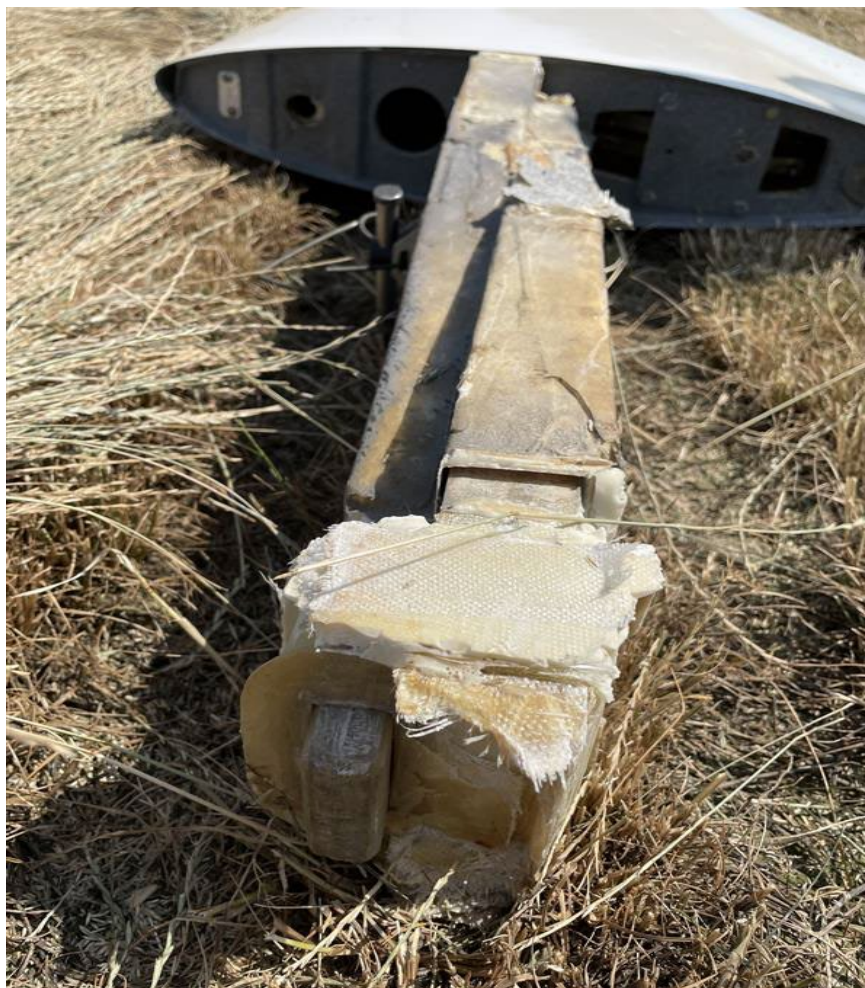
Photograph 4 - View of left wing root and spar still affixed to right wing root spar, held together by spar pin (Courtesy of FAA)
