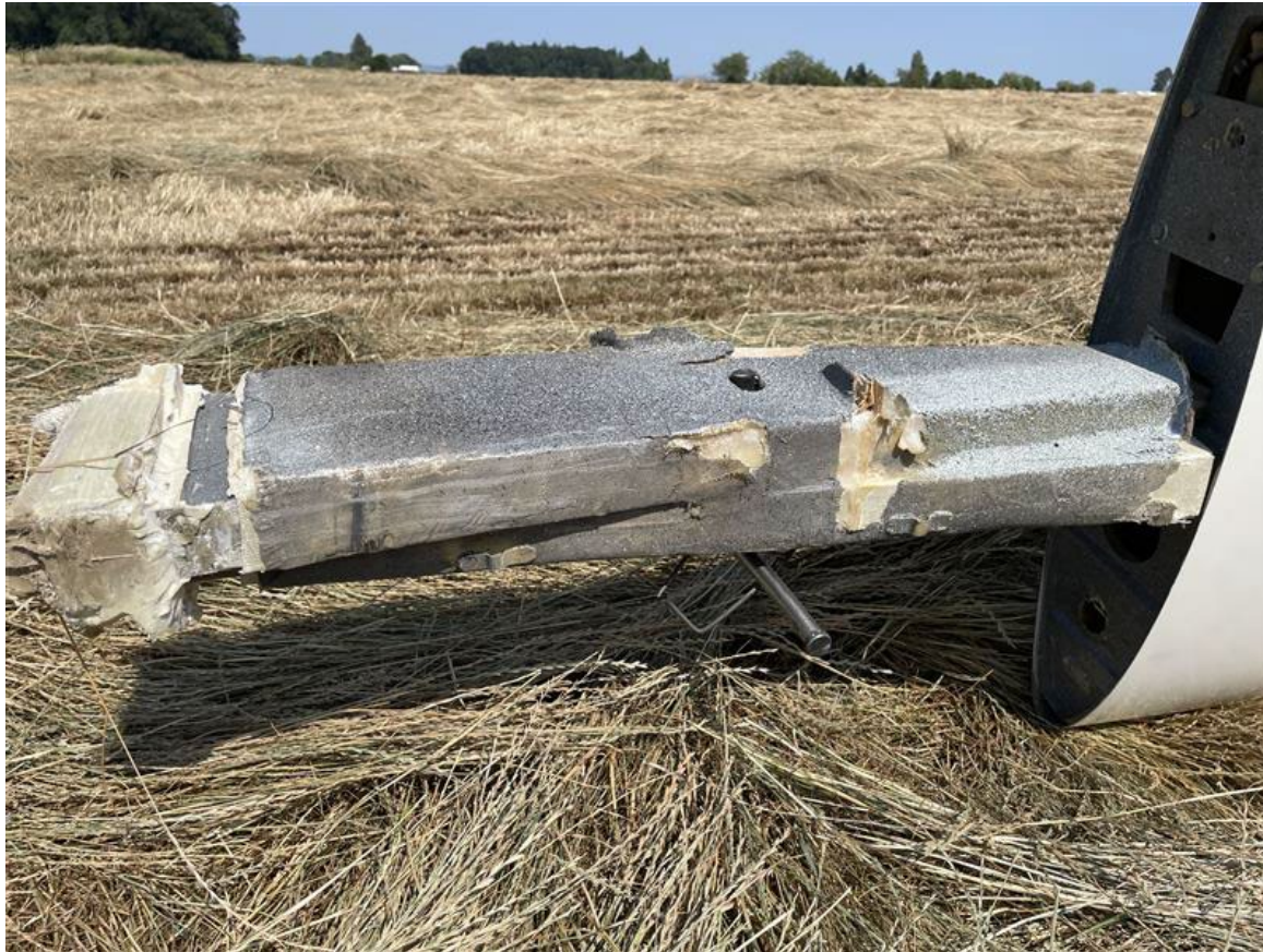
Photograph 5 - View of left and right wing spar assembly, and failure surface (Courtesy of FAA)
