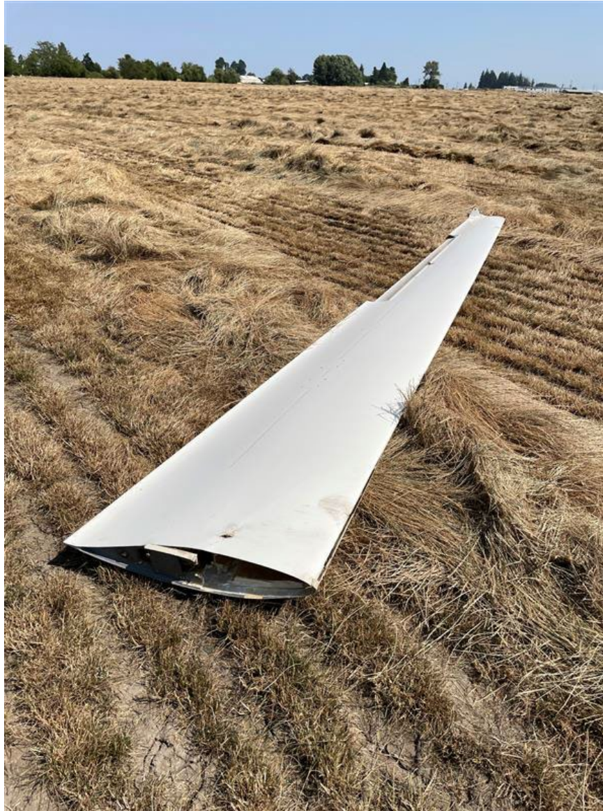
Photograph 3 - View of separated right wing without wing root spar (Courtesy of FAA)
