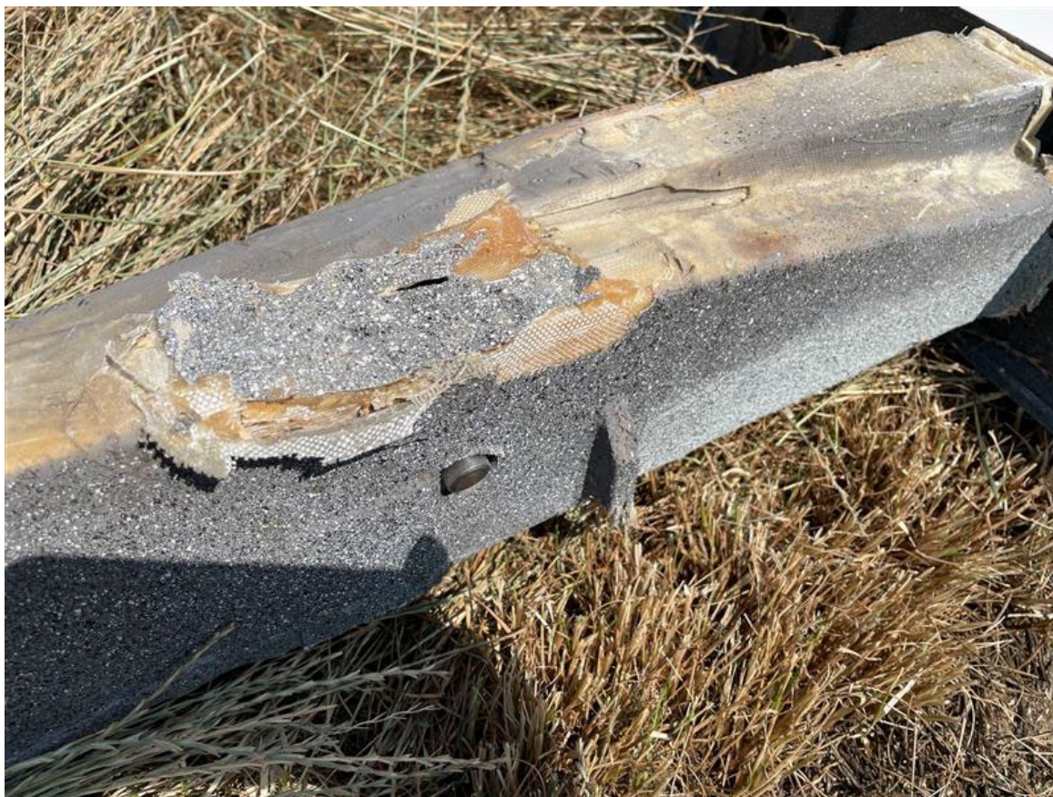
Photograph 6 - Aft view of spar pin connected through spar orifice (Courtesy of FAA)
