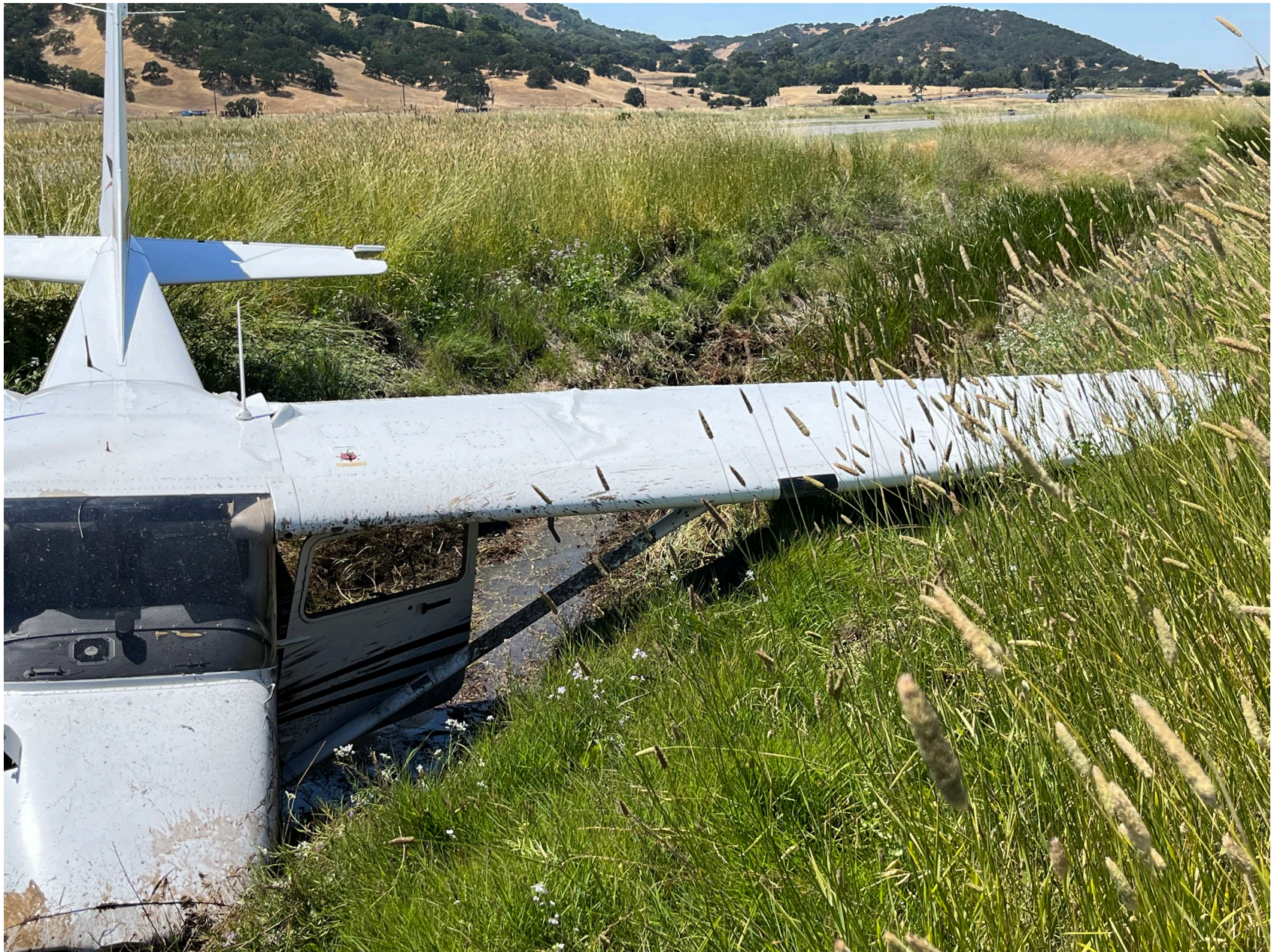
Photo 1 – View of left-wing damage (Photo courtesy of Pilot)
