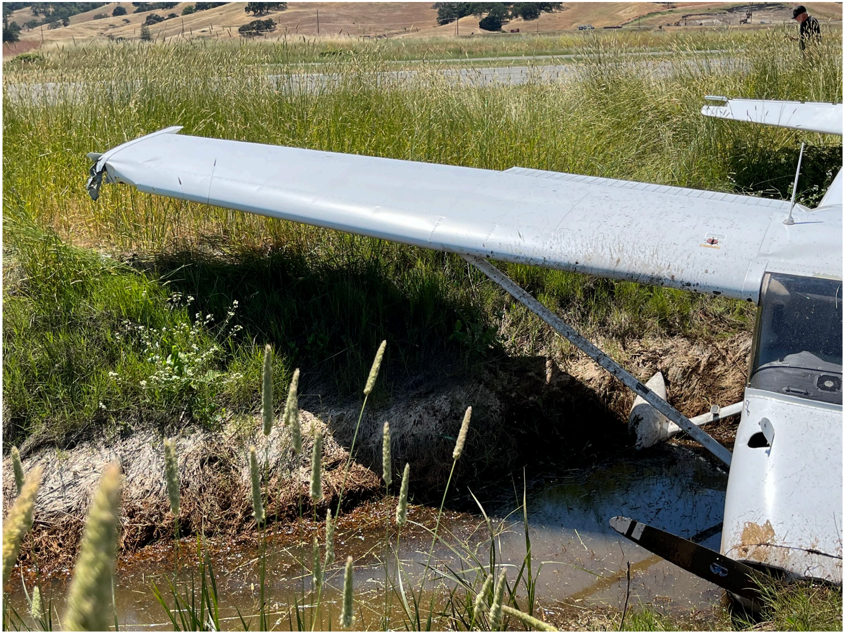
Photo 2 – View of right-wing damage (Photo courtesy of Pilot)
