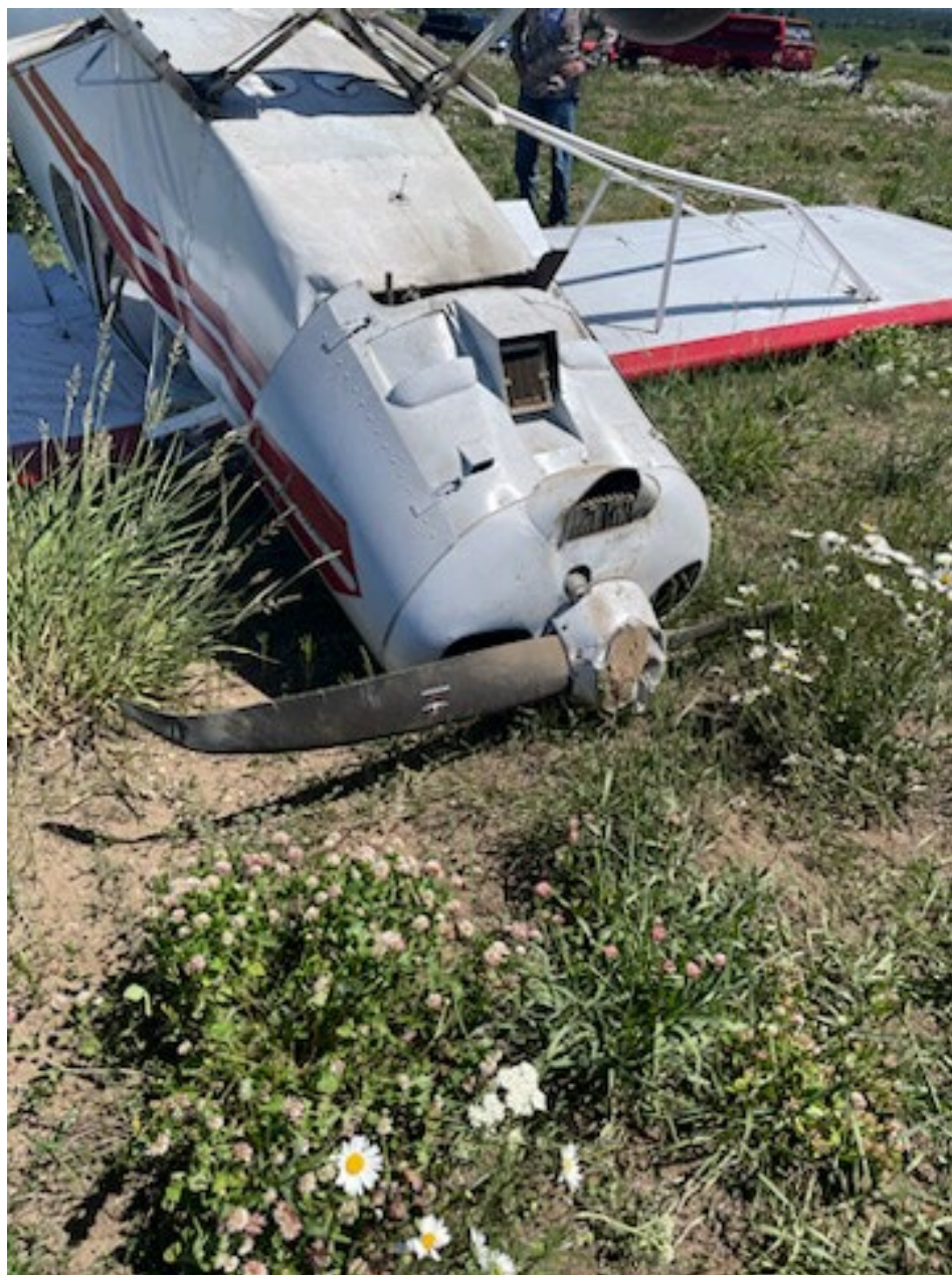
Photo 2 – View of right wing strut damage (courtesy of airpoart ops)
