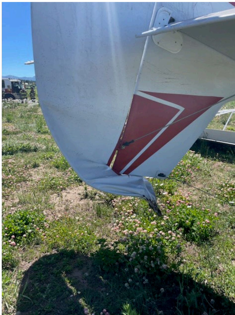
Photo 3 – View of rudder damage (courtesy of airport ops)
