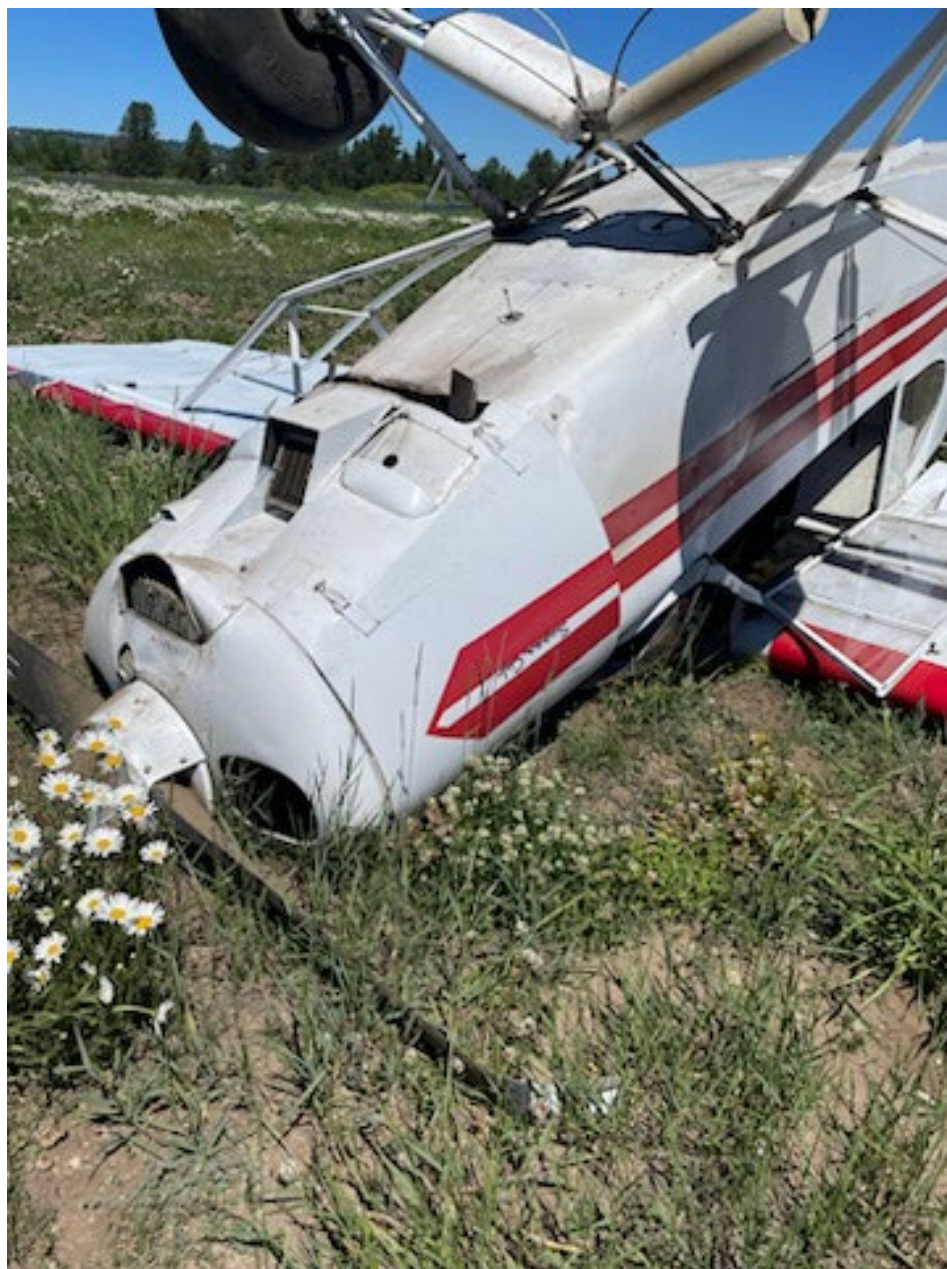
Photo 1 – View of left wing strut damage (courtesy of airport ops)
