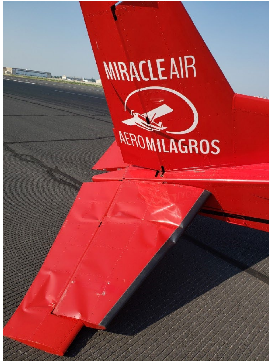
Photo 1 – View of Tail Damage (Source: Airport Operations)
