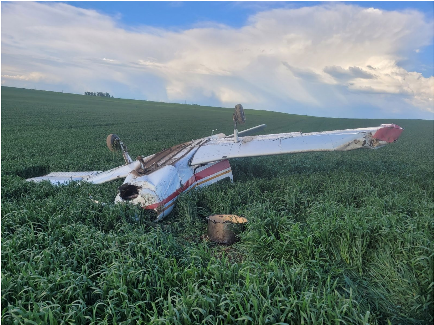
Photo 1 – View of damage to both wings (courtesy of LEO on scene)
