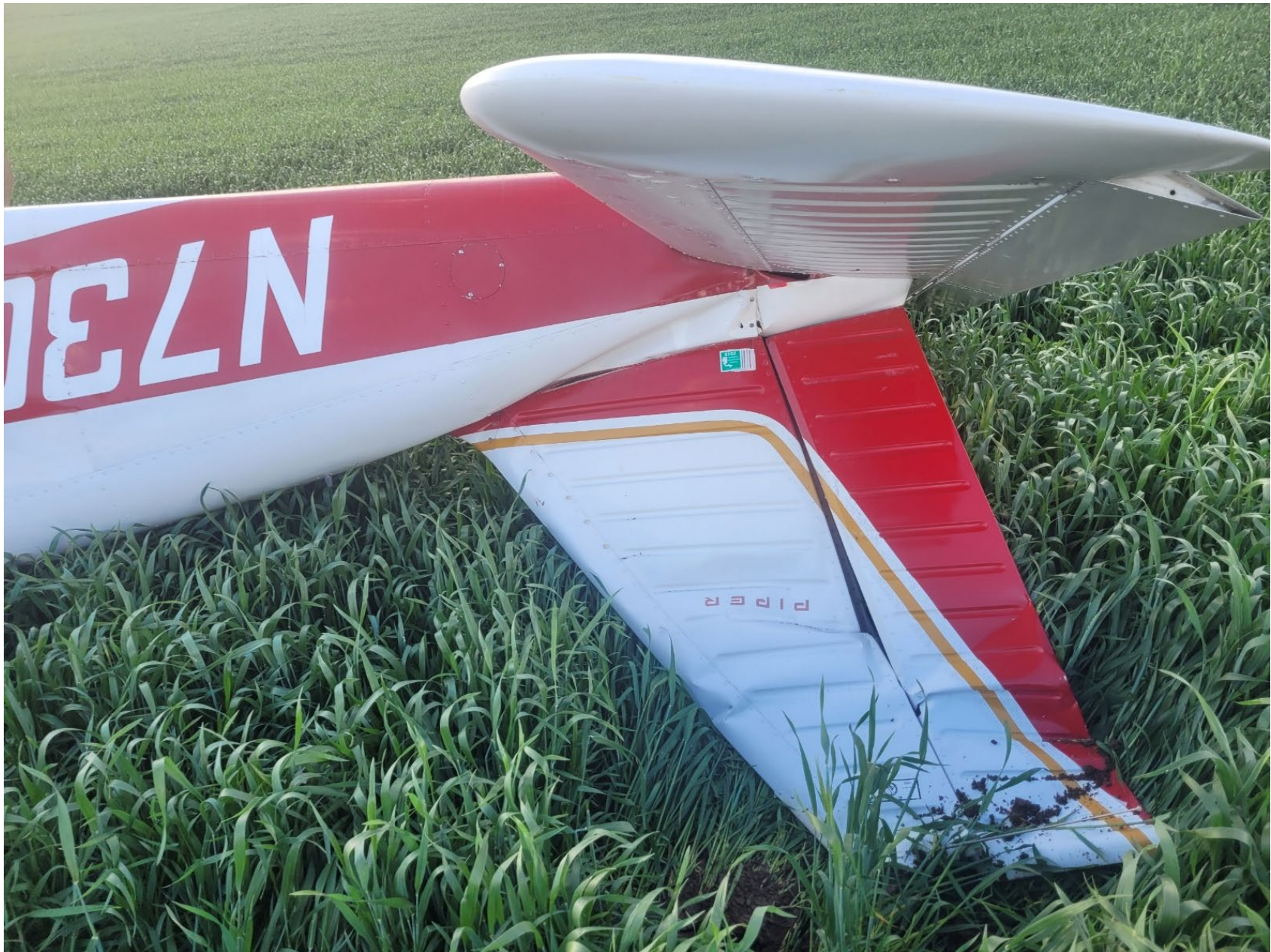
Photo 2 – View of damage to fuselage, vertical stabilizer, and rudder (courtesy of LEO on scene)
