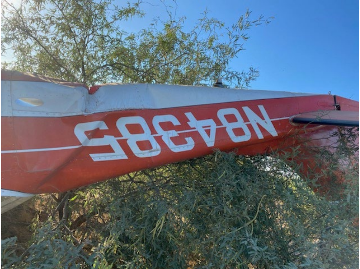
Figure 3. Close up view of the substantial damage to the tail cone area of the fuselage. Photo courtesy of the owner.
