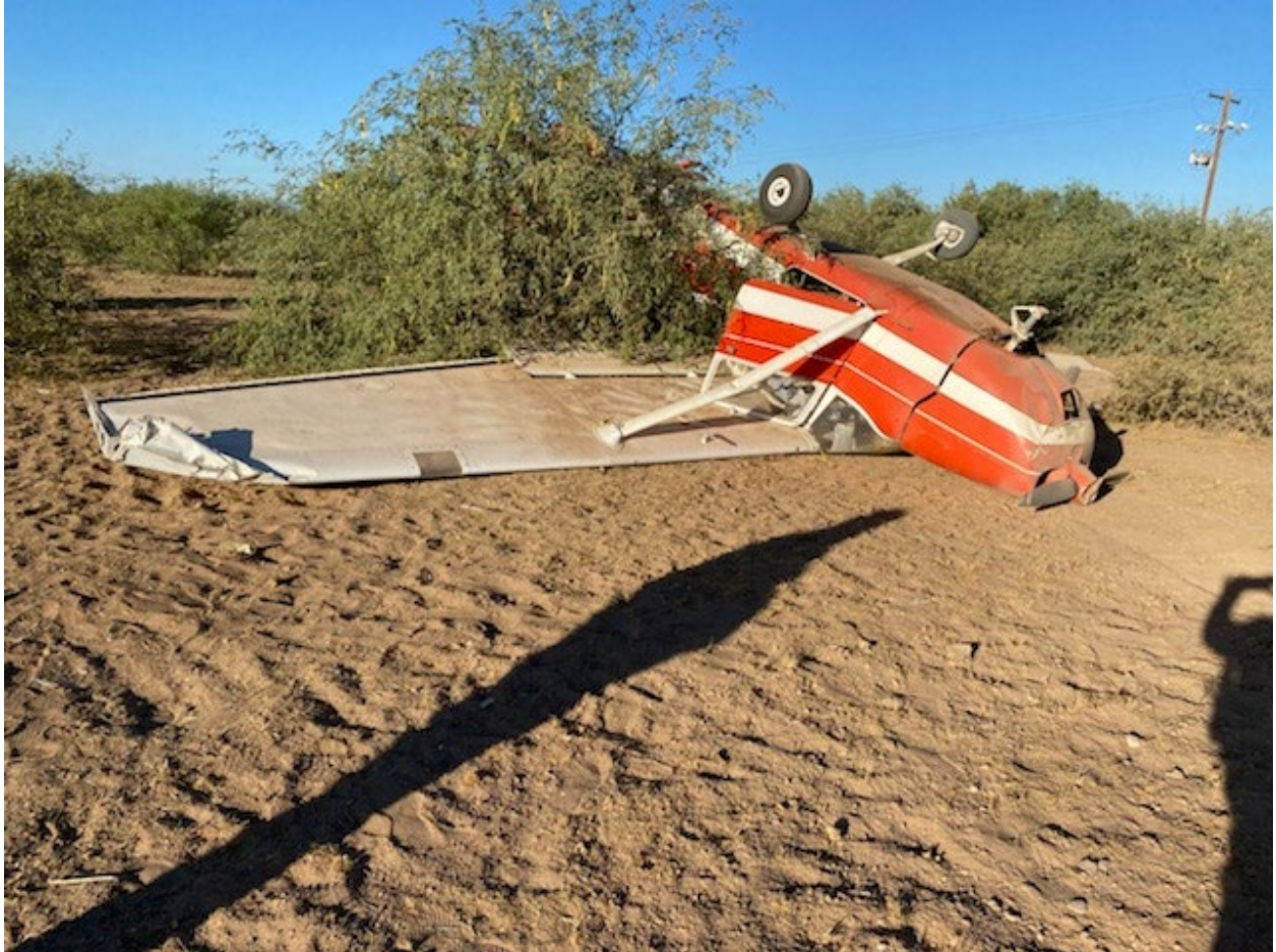
Figure 5. Left wing and wing strut damage. Photo courtesy of the owner.
