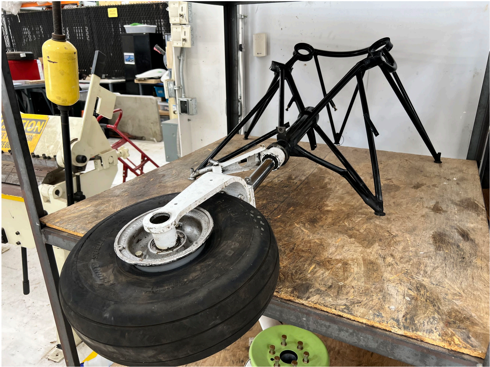
Photo 2 – View of Engine Mount Damage (Source: Flight School)
