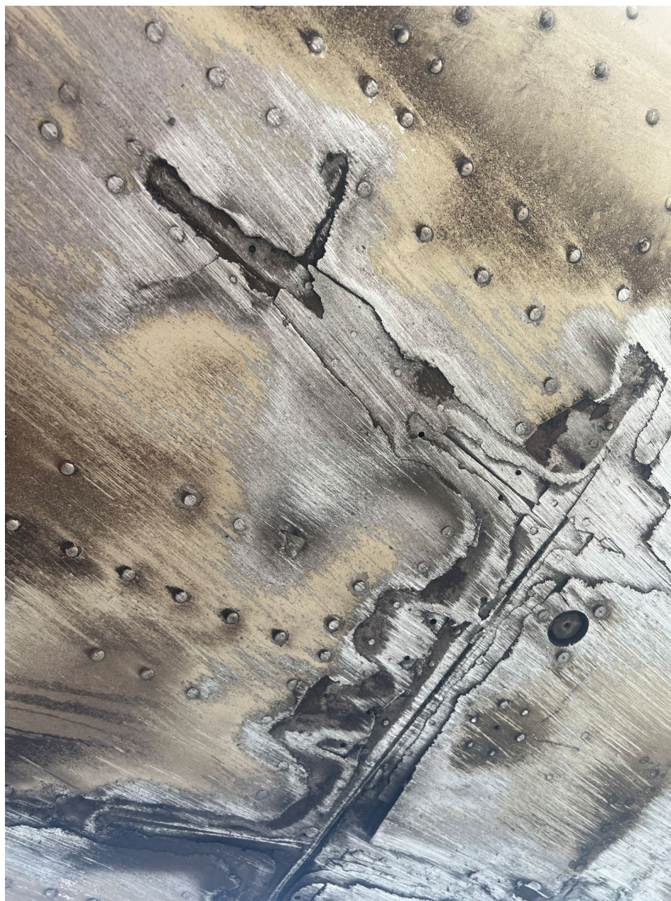
Photo 2 – Underside view of damage to the left and right keel beams. Photo courtesy of the pilot.
